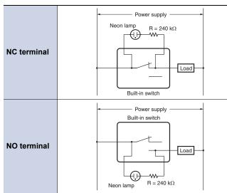
Note: If the wiring is as shown above, the operation of the respective parts will be as shown in the following table. The neon lamp is not wired when the Switch is delivered. Connect it as required.
