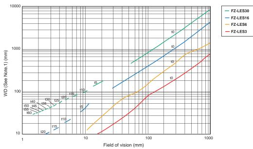
Note: The vertical axis represents WD, not installation distance.
