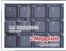
Seven times the field of vision is captured in 33.3 ms, the same time as for a 0.3megapixel Camera
