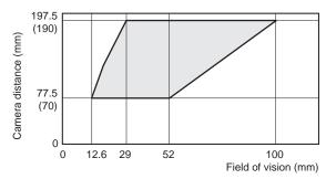
**Note:** The value in parentheses is for the camera installation distance when using an Intelligent Camera.
