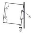
When mounting to a DIN Rail, lower the S82S onto the Rail until the Rail stopper clicks into space, hook section A over the edge of the Rail, and push in the direction of B.
