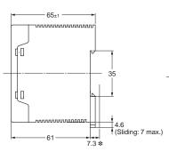
\* A distance of 7.3 mm is required between the model and the mounting surface when the mounting bracket provided with the model is used.
