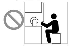
A person is between the sensor's detection zone and the hazardous zone of a machine.
