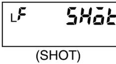
Shot output is the function that turns OFF a comparative output after a set interval after it turns ON.
