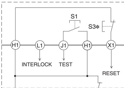
\* S3 If the switch is not necessary, connect between X1 and H1.
