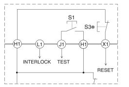
$\boldsymbol{*}$  S3 If the switch is not necessary, connect between X1 and H1.
