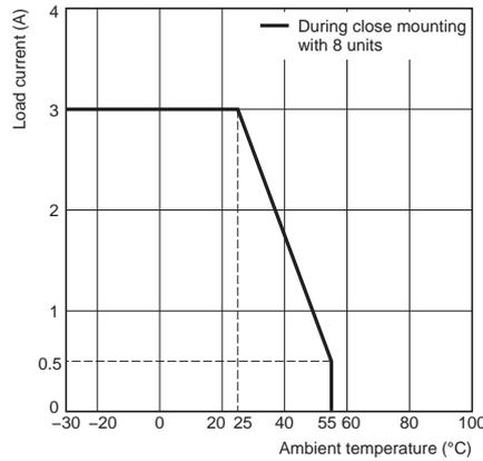
\* When eight or more are installed, install with 10 mm space between each.
