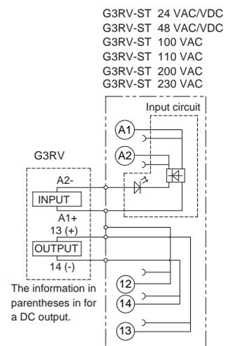
**Note:** For recommended ferrules, crimp tools, and types and gauges of wires, refer to 3. *Recommended Ferrules and Crimp Tools* on page 26.
