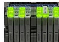
Visibility from the front is improved by a structure where the actual release lever lights and by expanding the light emission area.
