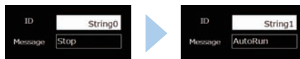
When the ID is specified by the variable, the text string is displayed according to the ID.
