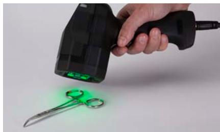
Direct Part Marks on highly reflective surfaces may be a challenge for some, but the V460's Intelligent Lighting and X-Mode algorithms make this as easy as point & click.
