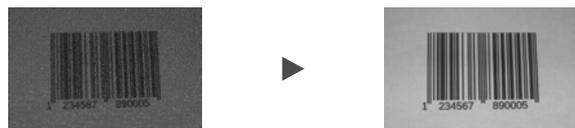
Automatic lighting adjustment to properly capture barcode Labels.
