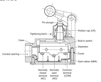
Note: The conduit thread indication has been changed from "PF1/2" to "G1/2" accompanying the JIS B 0202 revision. This changes applies only to the indication; thread sizes and pitches have not been affected.
