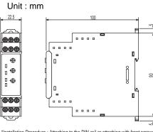
Installation Procedure : Attaching to the DIN rail or attaching with front screws Measurements for attachment with front screws
