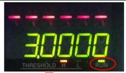
Hold down the **Mode switching** Key for two seconds.
