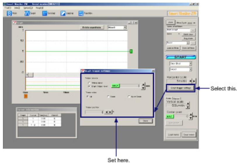
There are two types of graphic triggers, external signal triggers and self-triggers.
