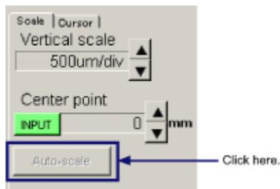
[Vertical Scale]/[Center Point] can be set manually.
