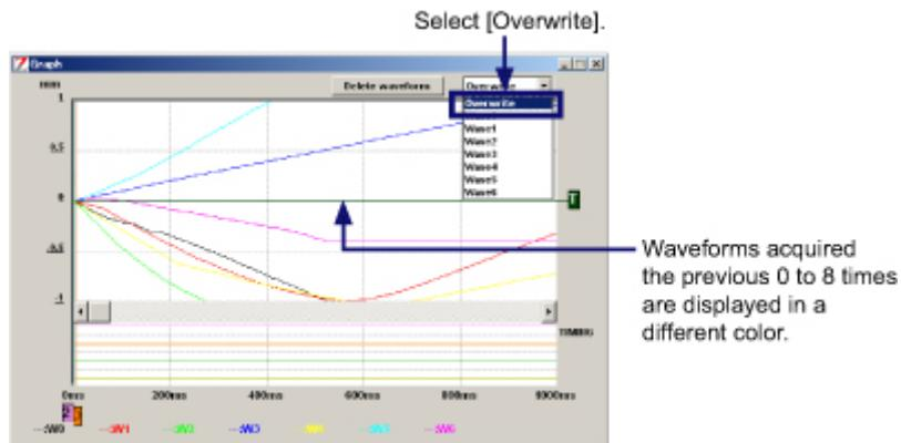
Clicking the **[Delete waveform]** button deletes all waveforms currently stored in the temporary memory.
