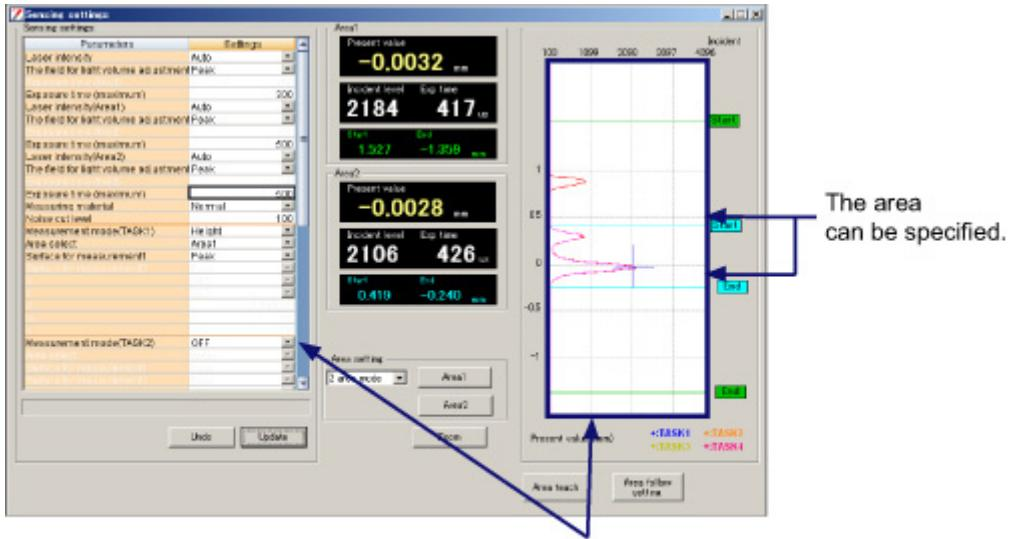
The sensing conditions can be set while confirming the incident level of the Sensor Head.
