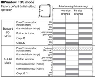
\*1 In IO-Link mode, output 2 can also be used in addition to communication output.
