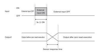
Note: When the power is turned off after zero reset is executed, zero reset is canceled. To retain the result of a zero reset, use the zero reset memory function.
