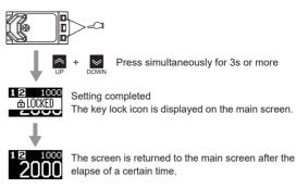
If buttons are operated in the key lock state, the key lock icon is displayed on the main screen.
