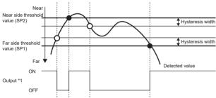
\*1. This is a graph when the output logic is N.O. It is inverted in the case of N.C.
