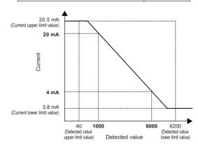
If Scaling High and Scaling Low are the same, the scaling setting is ignored and the operation is the same as with the initial values (Low: 50, High: 6000).
