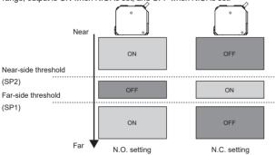
Note: Single point mode and window BGS mode perform the BGS operation, so they can be used regardless of whether there is a background, but window FGS mode cannot be used if there is no background
