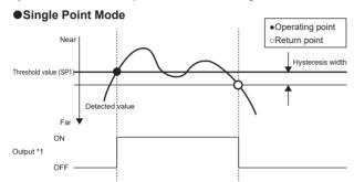
\*1. This is a graph when the output logic is N.O. It is inverted in the case of N.C.
