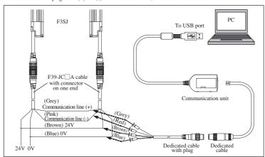
For information about the F3SJ wiring procedure, see the wiring diagram in the F3SJ User's Manual on the included CD-ROM.
