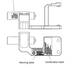
Label for laser radiation aperture
