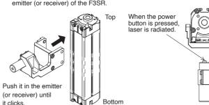
4. Perform coarse adjustment so that laser beam is radiated at the center of the top of the opposed receiver (or emitter). After adjustment, temporarily tighten the mounting bracket on top.
