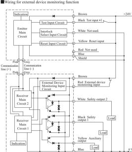
\*1 Emission is stopped : Short-circuited to 0 V to 1/2 Vs or open. Normal operation : Short-circuited to Vs-3 V to Vs.
