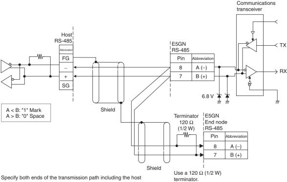
Specify both ends of the transmission path including the hos as the end node (that is, connect terminators to both ends). Use a terminating resistance of at least 54  $\Omega$ .
