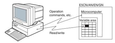
When accessing the variable area, the position of a variable in the variable area is specified with a word identifier, area number, and address in the area.
