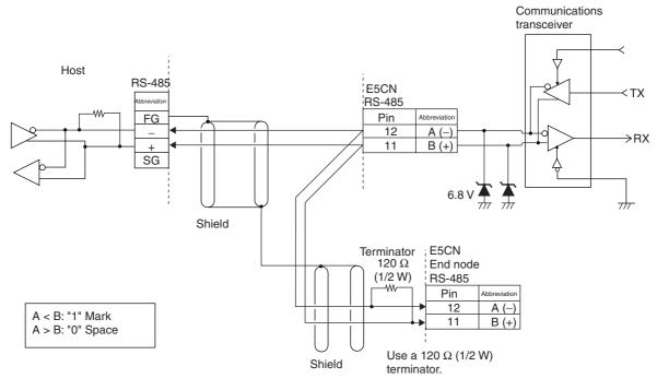
Specify both ends of the transmission path including the host as the end node (that is, connect terminators to both ends). Use a terminating resistance of at least 54  $\Omega$ .
