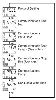
Note: Displayed only when the Protocol Setting parameter is set to CompoWay/F.
