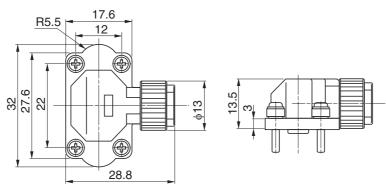
Angle plug model JN8FT04SJ1 (Japan Aviation Electronics) Socket contact model ST-TMH-S-C1B-3500-(A534G) (Japan Aviation Electronics)
