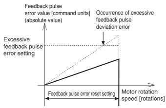
• When using feedback pulse error reset, make sure the feedback pulse error reset setting is set to a proper value. When the set value is extremely small, the protective function may not work to prevent any erroneous operation due to improper connection of the external encoder. Take sufficient care to ensure safety.
