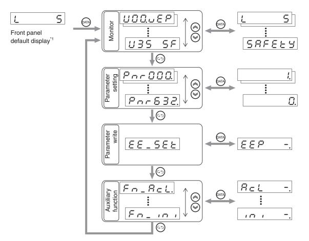
\*1. The display will be based on the Default Display (Pn528) setting after the power supply is turned ON.
