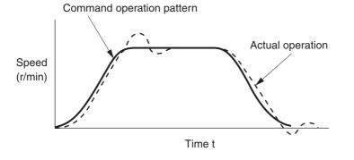
• If the position loop gain is low, positioning completion speed becomes slow.
