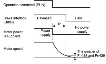
•"TB" in the above figure is the Brake Timing During Operation (Pn438) (set value × 1 ms) or the time until the motor rotation speed falls to the speed set for the Brake Release Speed Setting (Pn439) or lower, whichever is shorter.
