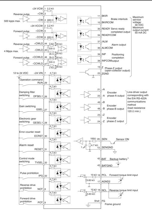
Control I/O Signal Connections and External Signal Processing for Position Control
