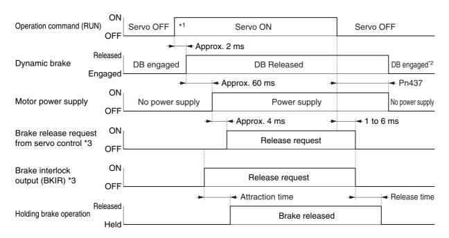
\*1. The servo does not turn ON until the motor rotation speed drops to approx. 30 r/min or below.
