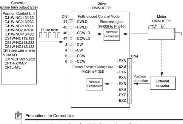
You cannot connect an external encoder with absolute encoder specifications.
