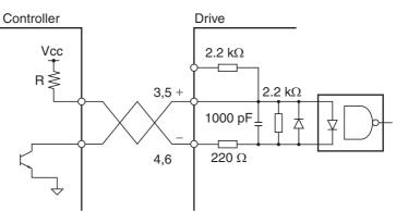
Select a Current Limit Resistor (R) appropriate for Vcc.
