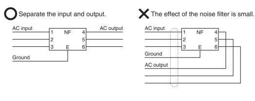
• Use twisted-pair cables for the power supply cables, or bind the cables.
