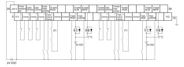
\*1. The XB and YB contacts are used to turn ON/OFF the electromagnetic brake. Note 1.Do not connect unused terminals.
