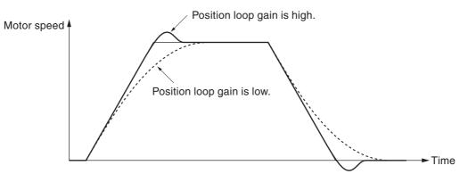
• If the speed loop gain and position loop gain are optimally set, the motor operation for the command will be delayed 2/Kp at acceleration and delayed 3/Kp at deceleration.
