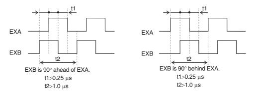
\*2. These are the feedback speeds from the external encoder at which Servo Drive can respond. Check the external encoder operation manual for its maximum output frequency. For example, the maximum speed when an external encoder with a resolution of 0.01  $\mu$ m is used for the serial communication type is 0.01  $\mu$ m × (400 × 10<sup>6</sup>) pps = 4.00 m/s. An overspeed error protection is generated, however, if the motor shaft rotation speed exceeds the maximum speed.
