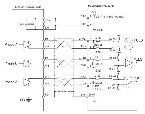
■ Serial Communications Type, Incremental Encoder Specifications (Pn323 = 1)
