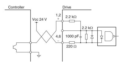
• External control power supply (200 kpps maximum) (+CW: 3, -CW: 4, +CCW: 5, -CCW: 6)
