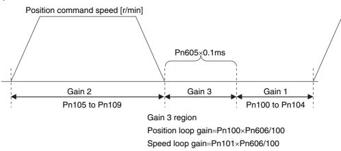
The gain 1 value is used for the speed loop integral time constant, speed feedback filter time constant, and torque command filter time constant.
