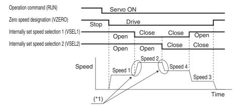
\*1. The acceleration time, deceleration time, and S-curve acceleration/deceleration time can be set using parameters (Pn312, Pn313, and Pn314).
