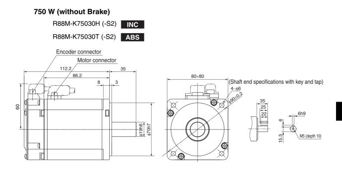
Models with an oil seal are indicated with O at the end of the model number. The motor dimensions do not change.
