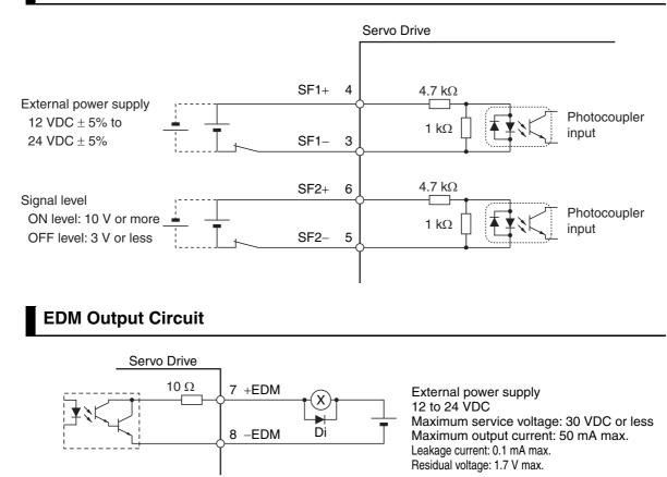
Di: Surge voltage prevention diode (Use a high-speed diode.)
