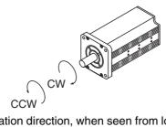
• Regarding the motor rotation direction, when seen from load-side axis, clockwise is referred to as CW and counterclockwise as CCW.
