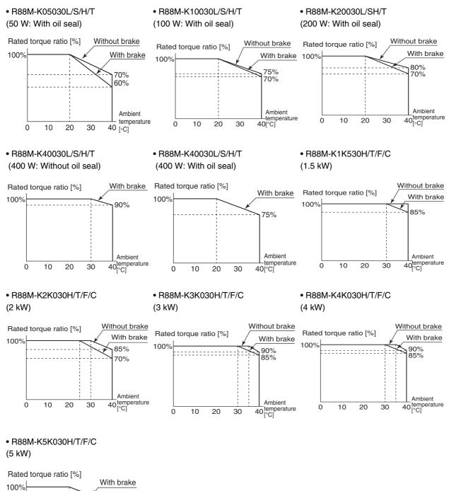
Use the following Servomotors in the ranges shown in the graphs below. Using outside of these ranges may cause the motor to generate heat, which could result in encoder malfunction.
