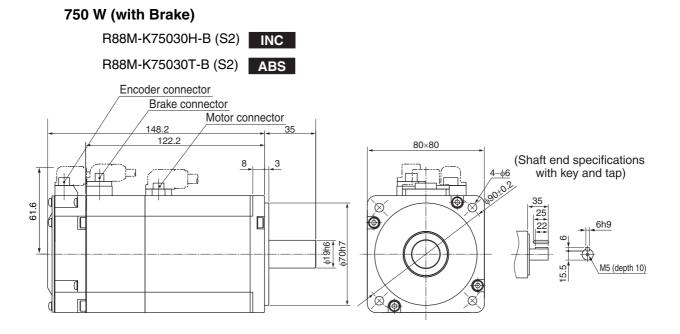
Note. The standard models have a straight shaft. Models with a key and tap are indicated with S2 at the end of the model number.
