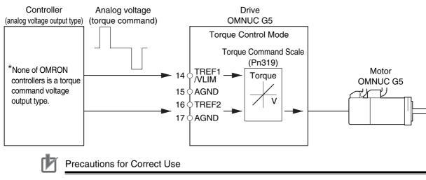
• If the motor speed is limited by the speed limit, the motor speed will be limited and will not reach the speed corresponding to the analog torque command.
