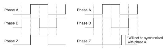
When the dividing ratio is multiple of 4
