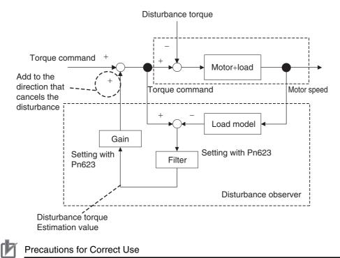
• If there is a resonance point below the cut-off frequency estimated by the disturbance observer or if a large amount of high-frequency elements is found in the disturbance torque, the disturbance observer may not be effective.
