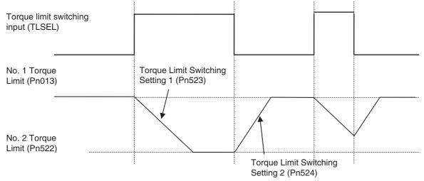
If the setting of No. 1 Torque Limit (Pn013) or No. 2 Torque Limit (Pn522) is changed from the front panel or CX-Drive, the rate of change setting will be ignored and the new torque limit value will be applied immediately.
