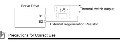
• Connect the thermal switch output so that the main circuit power supply is shut OFF when the contacts open.
