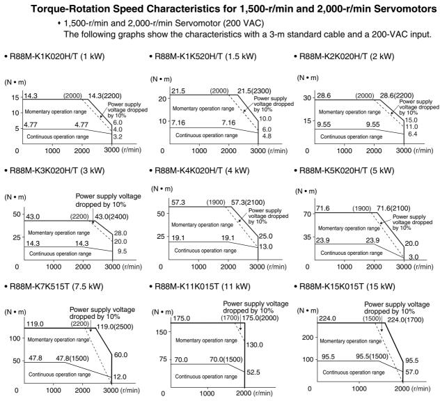
Note 1: The continuous operation range is the range in which continuous operation is possible. Continuous operation at the maximum speed is also possible. However, doing so will reduce the output torque.
