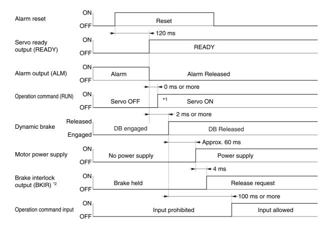
\*1. The servo does not turn ON until the motor rotation speed drops to approx. 30 r/min or below.
