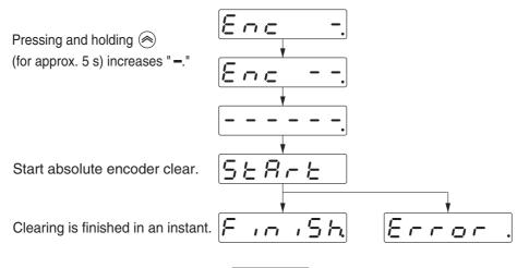
Note.  $\boxed{\mathcal{E} \ r \ r \ o \ r}$  will be displayed if absolute encoder clear is performed on an incremental encoder.
