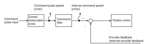
\*4. Position error and feedback pulse error come in 2 types, encoder unit/external encoder unit and command unit. Encoder unit/external encoder unit will be an error of position control input section and command unit will be an error of command pulse input.
