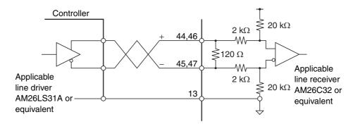
• The shielded twisted-pair cable should not exceed 10 m in length.
