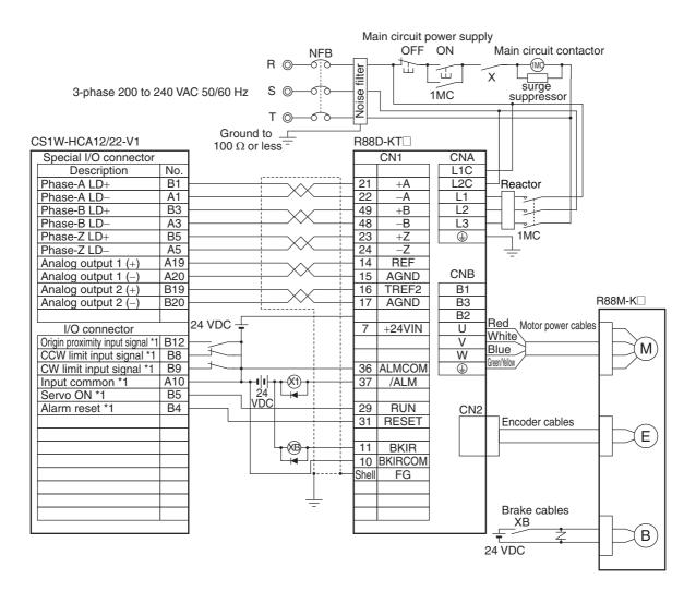
\*1. The I/O signals for the HCA12/22 depend on the allocations in the Internal Memory area. Change the wiring according to the allocations.
