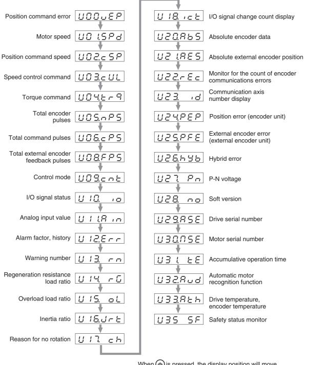
When () is pressed, the display position will move in the direction of the arrow.
