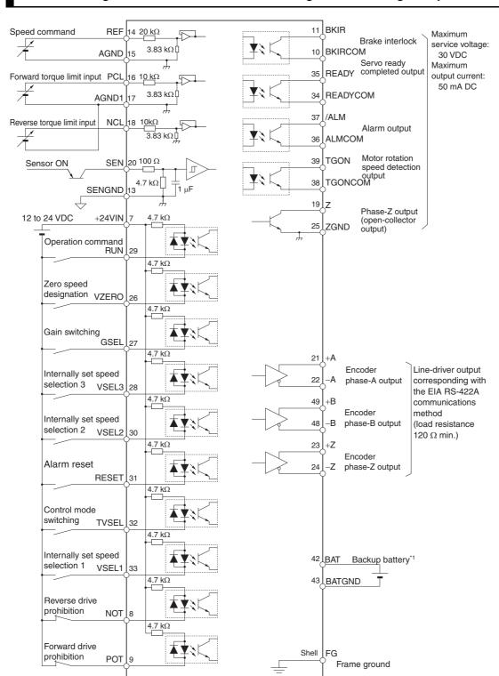
Control I/O Signal Connections and External Signal Processing for Speed Control
