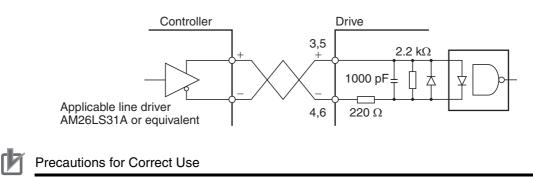
• The shielded twisted-pair cable should not exceed 10 m in length.
