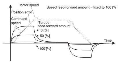
Torque feed-forward can reduce the position error in a range of constant acceleration/ deceleration.
