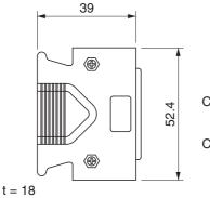
Connector plug model 10150-3000PE (Sumitomo 3M) Connector case model 10350-52A0-008 (Sumitomo 3M)
