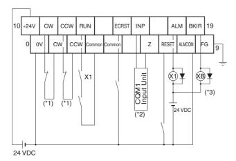
\*1. If this signal is input, the output pulse from the CQM1 will be input to the high-speed counter.
