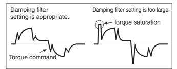
When the Damping Frequency 1 (Pn214) is set, reduce the setting if torque saturation occurs or increase the setting to increase operation speed. Normally 0 is set.
