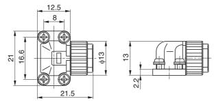
Angle clamp model JN6FR07SM1 (Japan Aviation Electronics) Connector pin model LY10-C1-A1-10000 (Japan Aviation Electronics)
