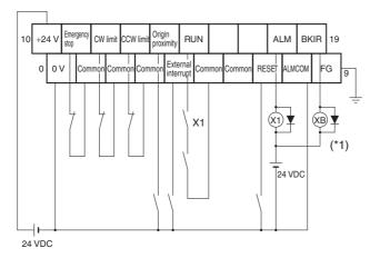
\*1. The XB contacts are used to turn ON/OFF the electromagnetic brake. Note 1.Do not connect unused terminals.
