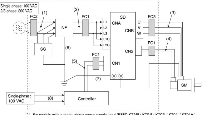
\*1. For models with a single-phase power supply input (R88D-KTA5L/-KT01L/-KT02L/-KT04L/-KT01H/-KT02H/-KT04H/-KT08H/-KT10H/-KT15H), the main circuit power supply input terminals are L1 and L3.
