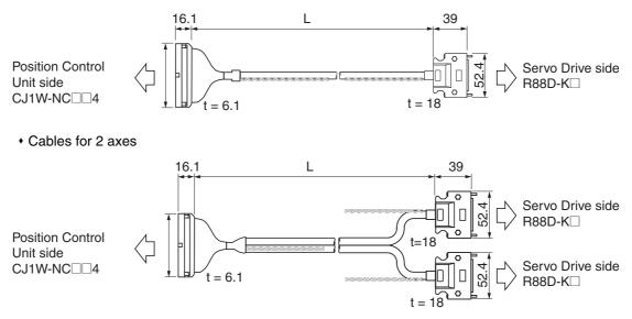
Cable for line-driver output for 1 axis
