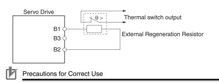
• Connect the thermal switch output so that the main circuit power supply is shut OFF when the contacts open.
