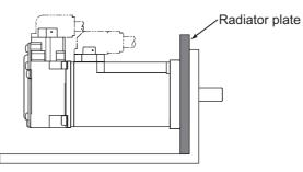
• The temperature rise depends on the mounting part materials and the installation environment. Check the actual temperature rise by using a real Servomotor.
