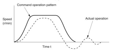
• If the speed loop gain is high, vibrations are more likely to occur. Vibration or resonance may not disappear.
