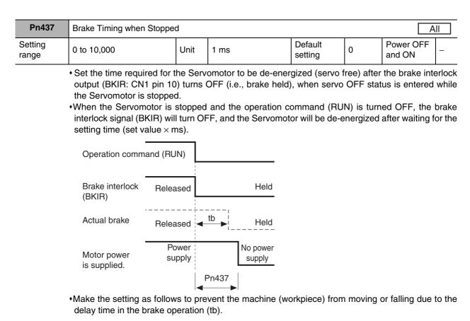
Brake timing when stopped (set value  $\times 1 \text{ ms}$ )  $\geq \text{tb}$
