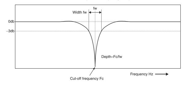
If machine resonance occurs, use this notch filter to eliminate resonance.
