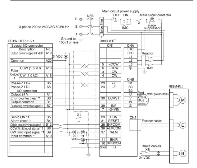
\*1. The I/O signals for the HCP22 depend on the memory allocations in the Internal Memory area. Change the wiring according to the allocations.
