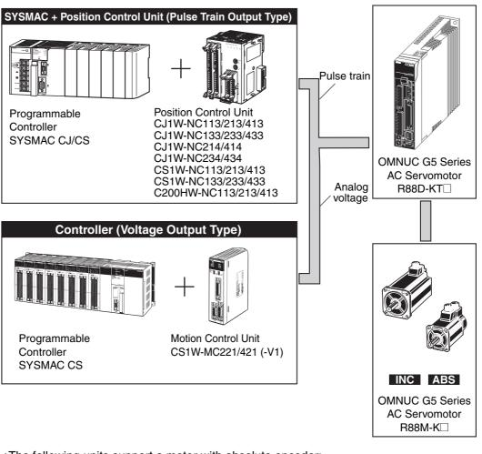
•The following units support a motor with absolute encoder: CJ1W-NC214/414 CJ1W-NC234/434 CS1W-MC221/421 (-V1)
