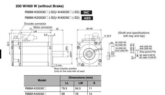
Models with an oil seal are indicated with O at the end of the model number. The motor dimensions do not change.
