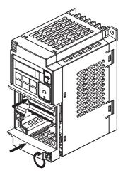
**5** Push the CompoNet Communications Unit into the previous location of the CompoNet Communications Unit cover until it clicks into place.
