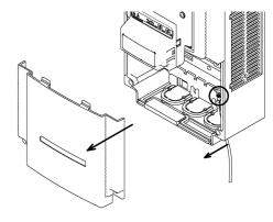
Remove the grounding cable of inverter.
