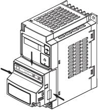
For inverters up to 4.0 kW, loosen the screws of the terminal block cover to remove the cover.
