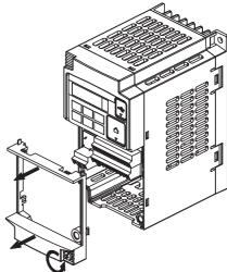
Connect the CompoNet Communications Unit's grounding cable to inverter with a mounting screw.
