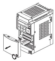
**2** For inverters up to 4.0 kW: Loosen the screws of the terminal block cover.
