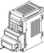
6 Press down on the indicated corner of the Compo-Net Communications Unit housing to ensure proper connection of the CompoNet Communications Unit connector.
