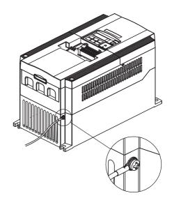
If removed in Step 2, reinstall the terminal cover and tighten the screw.
