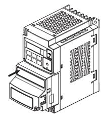
7 Check that there is no gap between the top edges of the CompoNet Communications Unit and the inverter casing.
