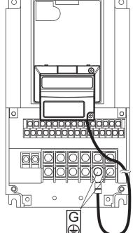
**9** Reinstall the terminal cover and tighten the two screws to fix it in position.
