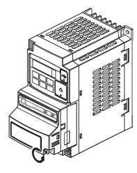
**2** Pull the CompoNet Communications Unit straight out of the inverter while pushing down on the indicated sides to release the snap-fits.
