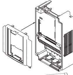
4 Connect the connector of inverter connection PCB of CompoNet Communications Unit to the connector of inverter.
