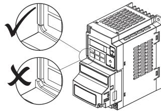
8 Secure the CompoNet Communications Unit in place to the inverter with the mounting screw.
