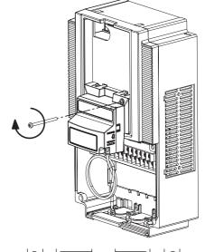
**8** Connect the grounding cable of the CompoNet Communications Unit to the ground terminal of the inverter.
