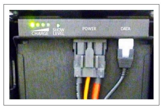
Figure 10-11. Battery Cable Connectors
