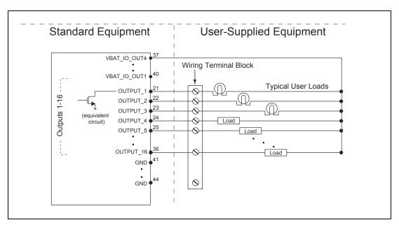
Figure 6-7. Typical Digital Output Wiring Example
