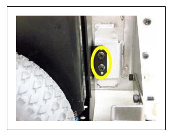
Figure 10-18. Mounting Screws at Bottom-Right of Drive Assembly
