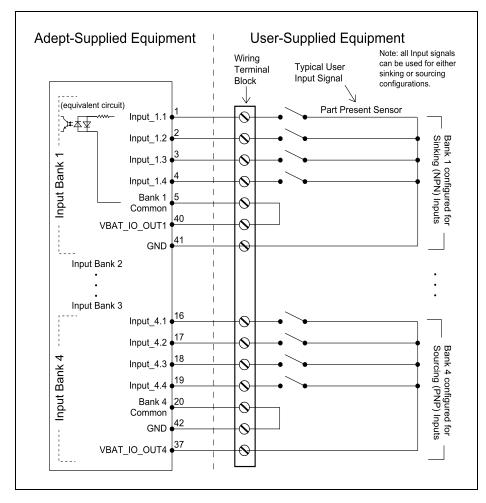
Figure 6-6. Typical Digital Input Wiring Example
