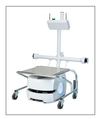
Figure 1-2. Cart and LD Platform Cart Transporter, Coupled
