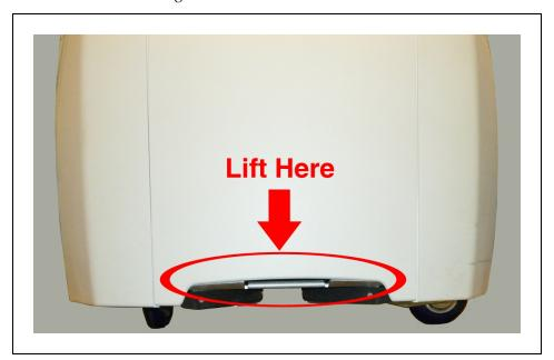
Figure 10-5. Bottom of Inner Rear cover. Lift from the frame, not the cover.
