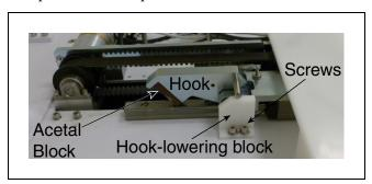
Figure 10-15. Hook-lowering Block and Screws
