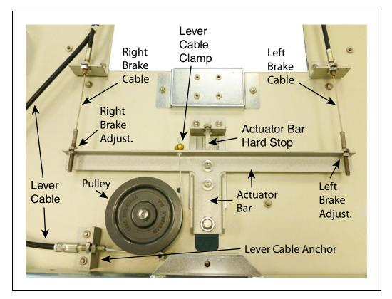
Figure 3-25. Internal Brake-Release Mechanism
