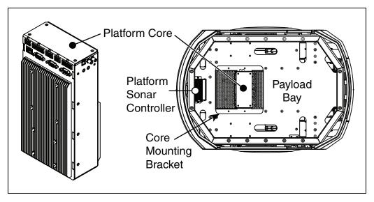
Figure 10-3. Location of Parts in the Payload Bay
