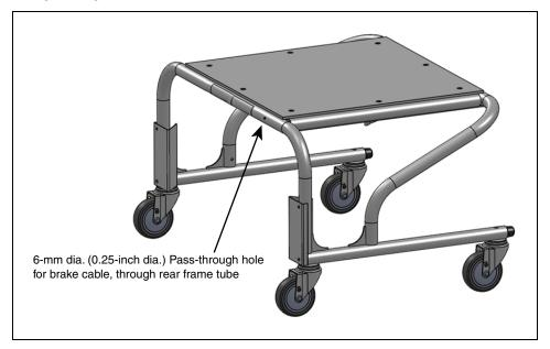
Figure 3-23. Thru-hole for Brake-release Cable
