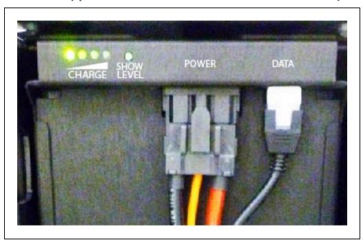
Figure 3-14. Battery Cable Connectors
