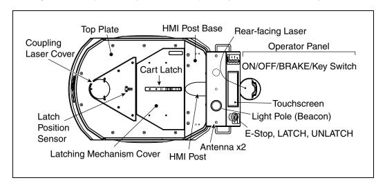
Figure 10-2. Top View of an LD Platform Cart Transporter, Side Laser Support Tubes Removed
