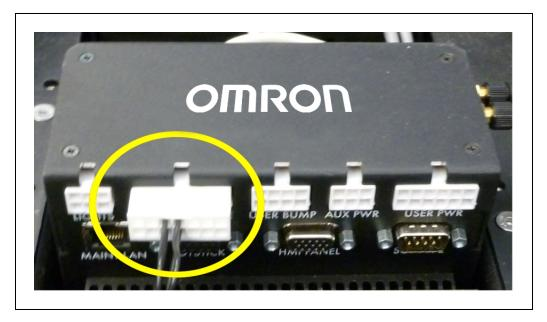
Figure 6-10. E-Stop Jumper on Platform Core
