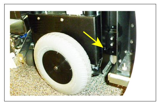
Figure 3-8. Wheel Pin Hole Location
