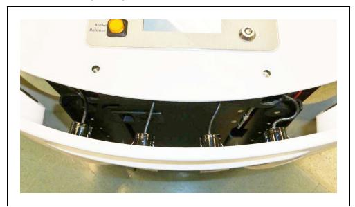
Figure 10-8. Sonar Leads, with Connectors Still in Chassis
