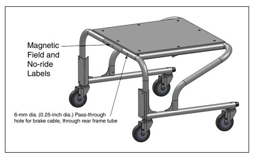
Figure 10-7. Magnetic Field/Implant, and No Riding Labels on Cart
