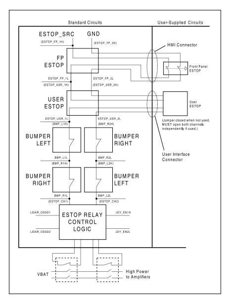
Figure 6-11. E-Stop Chain Diagram
