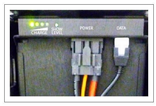
Figure 8-2. Battery LEDs, Push-Button, Power Cable, and Data Cable
