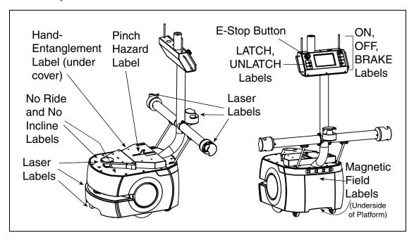
Figure 10-6. Locations of Labels on LD Platform Cart Transporter
