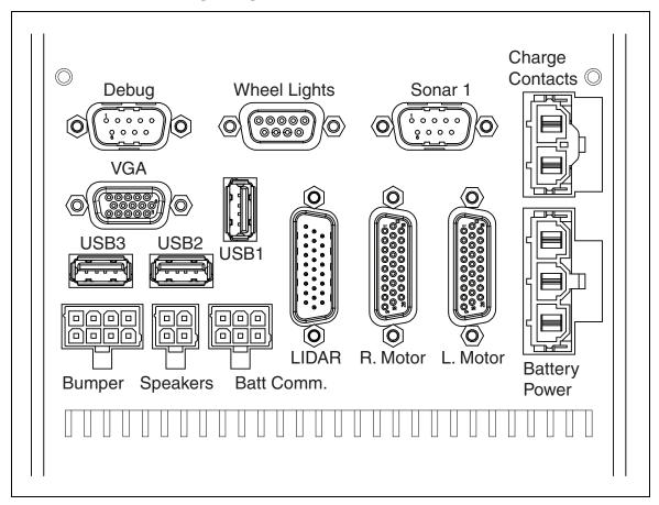
Figure 6-12. Internal Connectors on the LD Platform Core (Front)
