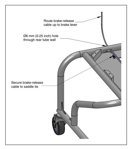
Figure 3-24. Thru-holes for Brake-release Cable, Plate Removed
