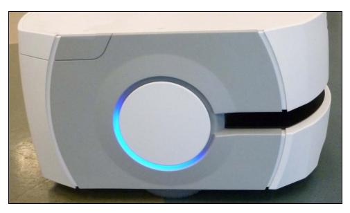
Figure 10-10. Right Side Cover, Showing Even Gaps at Edges
