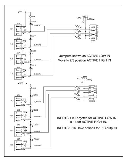
Figure 6-3. Input Schematic
