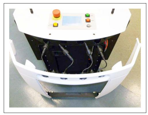
Figure 10-9. Sonar Connectors, with Connectors Exposed
