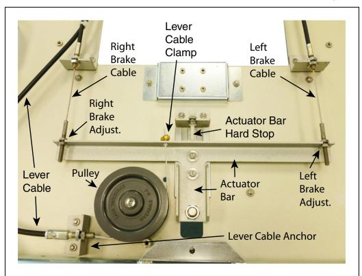
Figure 10-22. Internal Brake-Release Mechanism
