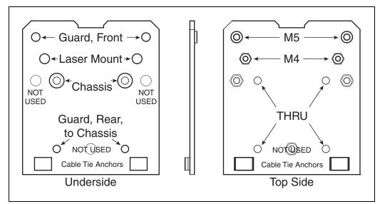
Figure 10-13. Mounting Plate for Low Front Laser and Guard
