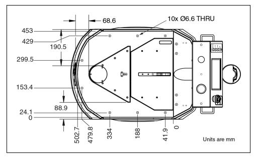
Figure 11-2. Coupling Plate Dimensions, Arms Removed
