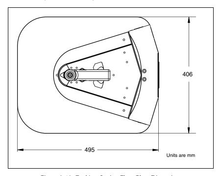
Figure 3-19. Docking Station Floor Plate Dimensions
