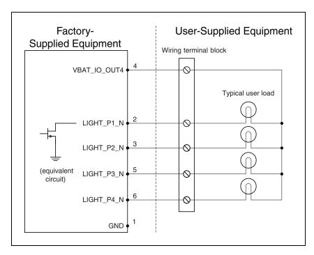
Figure 6-9. Sample Light Pole Diagram
