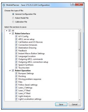
Figure 7-3: Save Robot Configuration window
