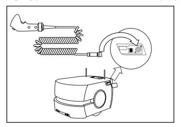
Figure 3-11: Connecting the joystick to the robot
