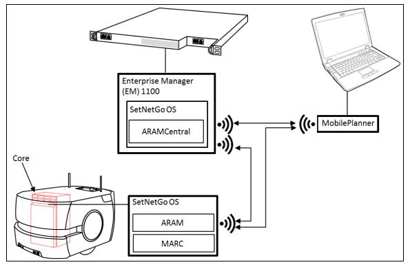
Figure 1-3: Components working together
