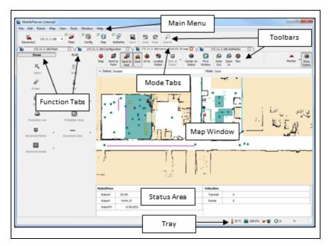
Figure 4-2: The MobilePlanner Interface (Example)
