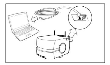
Figure 3-2: Ethernet Connection
