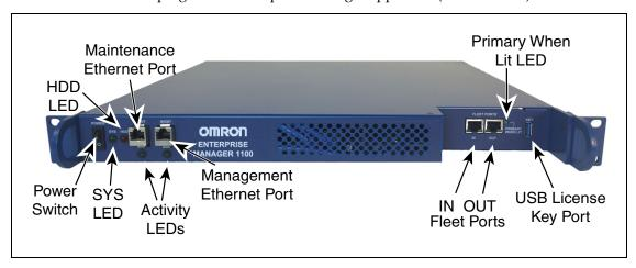
Figure 5-1. Front Connectors and Indicators
