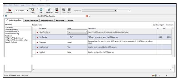
Figure 5-5. MobilePlanner, ARCL Server Setup Screen
