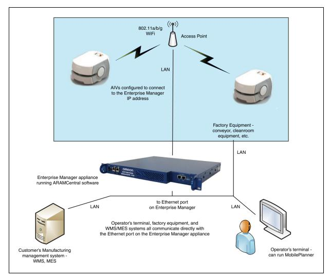
Figure 1-1. Main Components of an Enterprise Manager 1100 Installation
