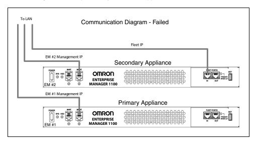
Figure 5-8. Sample Autosynchronized Application Communication, Primary Failed
