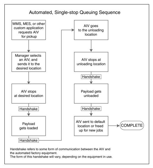
Figure 6-2. Fully-automated Queuing Cycle
