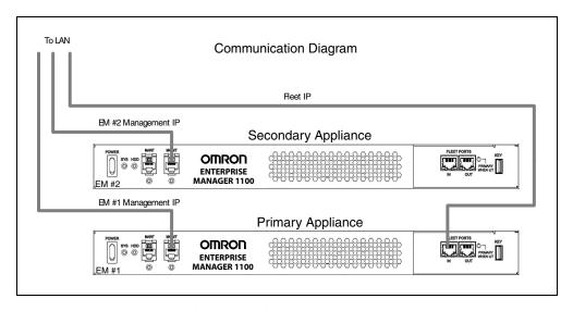
Figure 5-7. Sample Autosynchronized Application Communication
