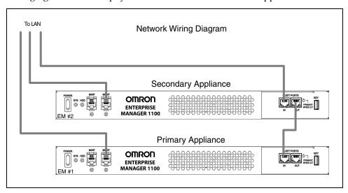
Figure 5-6. Sample Autosynchronized Network Connections
