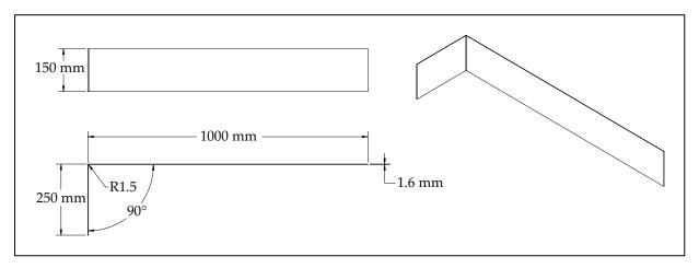
Figure 10-10. Standard Target
