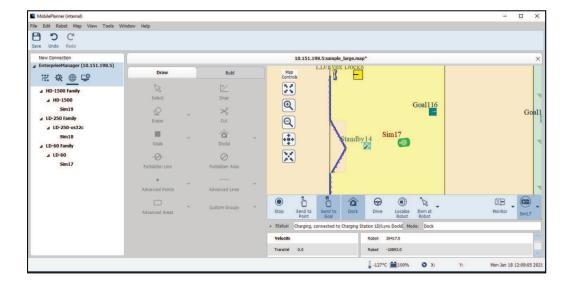
Figure 6-1. MobilePlanner, Manual Override ON
