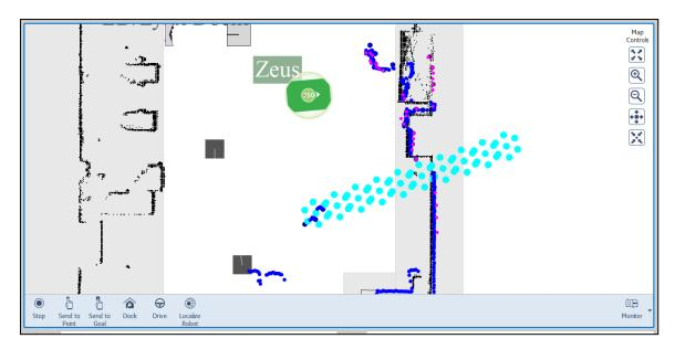
Figure 11-7. Path Projected by Two Moving Legs of a Walking Person (Shown in Cyan)
