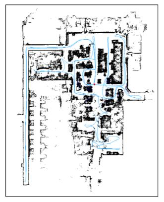
Figure 7-1. Example scanning path with ample looping around rooms
