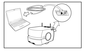
Figure 4-3. Maintenance Port Connection, LD-60 and LD-90
