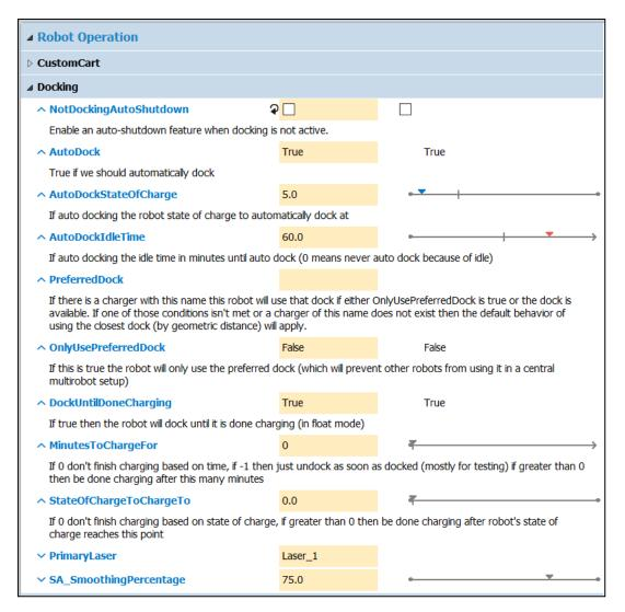
Figure 7-12. MobilePlanner Config - Robot Operations tab, Docking Parameters
