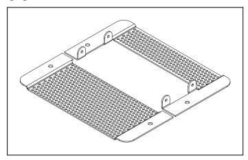
Figure 14-10. Core Mounting Bracket
