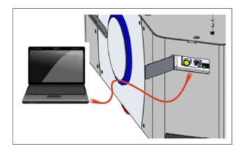
Figure 4-4. Maintenance Port Connection, LD-250
