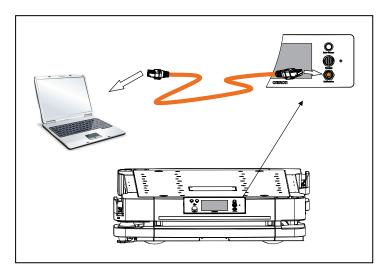
Figure 4-5. Maintenance Port Connection, HD-1500
