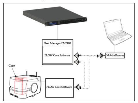
Figure 14-2. FLOW Core Fleet Topology with EM2100
