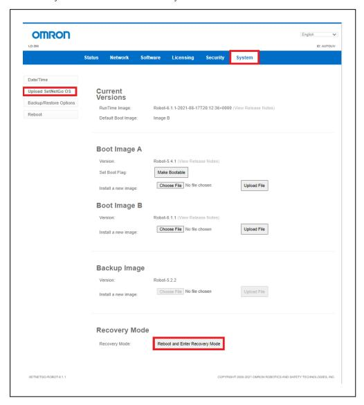
Figure 8-15. Reboot and Enter Recovery Mode Button
