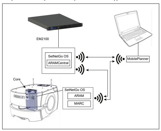
Figure 1-1. Components Working Together (LD-60 AMR Shown)
