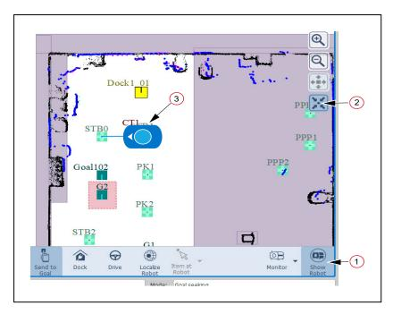
Figure 6-2. AMR on Map (Show Robot ON)
