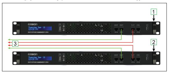
Figure 3-1. Cabling for an EM2100 Fleet Manager Pair
