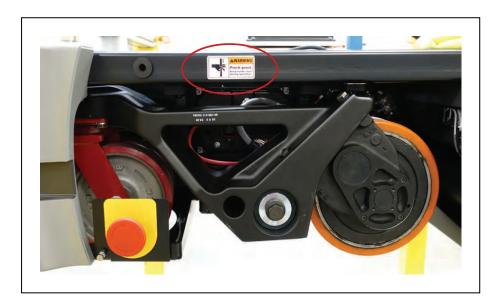
Figure 2-6. Side Skin Removed - Exposing Motor and Motor Assemblies
