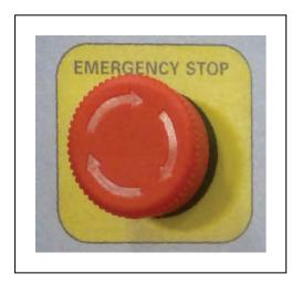
Figure 2-5. E-Stop Button on the Operator Panel
