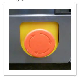
Figure 2-4. E-Stop Button on the Platform
