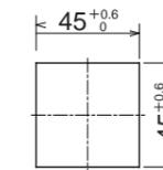
When installing the Products adjoining each other, secure enough space between the products. Reference interval: 60mm (top/bottom/left/right directions) For any product, it is the interval from the center.
