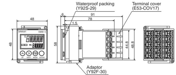
Mount the Product such that the display can be seen properly from the front. To fix the Product to the panel, use the attached adapter. Push the adapter from the terminal side until it hits the panel, and then tighten the panel temporarily. Tighten the fixation screw of the adapter with specified torque. Fixation screw tightening torque : 0.29~0.39N·m
