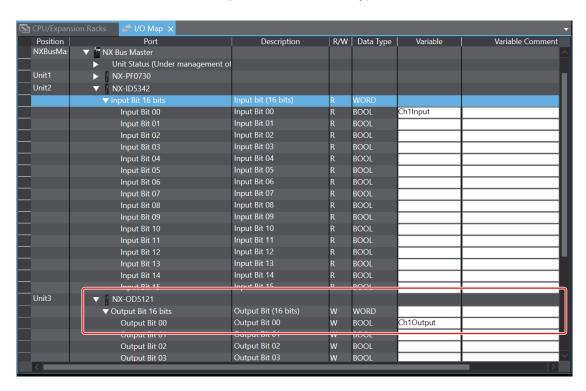
Set the network exposure of the abnormal status output variable Ch1Output to Publish Only. Open the settings screen from the left tab: **Programming**  $\rightarrow$  **Data**  $\rightarrow$  **Global Variables**.
