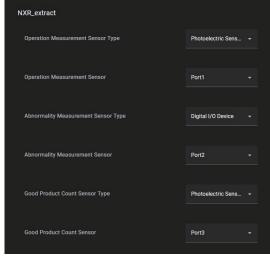
\*1 Even when not using the Good Product Count Sensor, please select "Photoelectric Sensor E3AS" for Good Product Count Sensor Type and select the "Port" where the Operation Measurement Sensor is connected.
