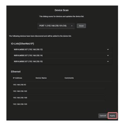
You will return to the *Device List Screen*. Confirm that the devices have been updated. The IP address of the slave-side Data Flow Controller will be shown at the bottom under the Ethernet section.
