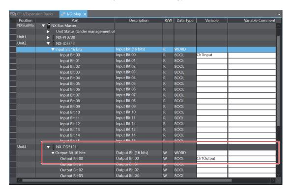
Set the network exposure of the abnormal status output variable Ch1Output to Publish Only. Open the settings screen from the left tab: **Programming** → **Data** → **Global Variables**.
