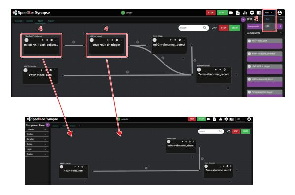
5 From the tab on the left, select **EtherNet/IP Collector** and place it.
