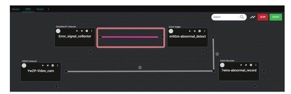
**9** Connect the output port on the right side of the created component to the input port on the left side of the *Event Recorder*.
