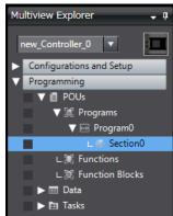
You can divide a ladder diagram into smaller units and set a name for each unit. This makes the program easy to understand and manage. The section can be moved and deleted.
