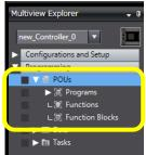
A POU (program organization unit) is a unit that is defined in the IEC 61131-3 and used to build the user program. There are three types of POUs: programs, functions (FUNs), and function blocks (FBs). FUNs and FBs that are reusable software components make programming easier.
