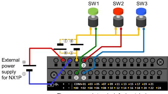
The power supply terminals for input devices do not have polarity
