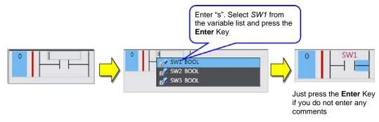
In the same way insert circuit parts as shown below.
