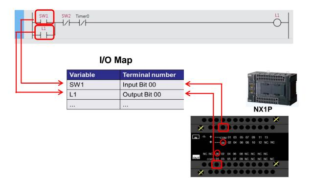
Variables used in the program are linked with actual I/O (input/output terminals of the NX1P in this example). You can change I/O assignments by simply changing the terminal number in the I/O Map. The benefit of programming with variables is that there is no need to change the program itself.
