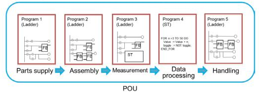
Two different programming languages, ladder diagram and ST, can be used. You can choose the appropriate language for each process and also program in ST within a ladder diagram program (inline ST).
