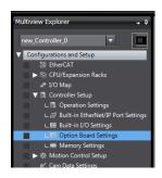
**2.** Select *NX1W-ADB21* (Analog Input Option Board) for the *Option board 1* parameter.
