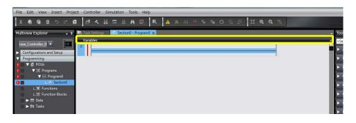
**3.** Register the variables used for inline ST as internal variables in the variable table.
