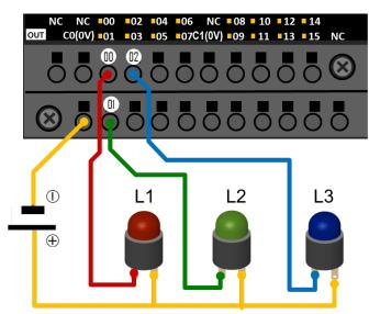
The power supply terminals have polarity
