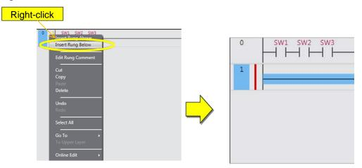
(3) Insert a program input in an OR structure
