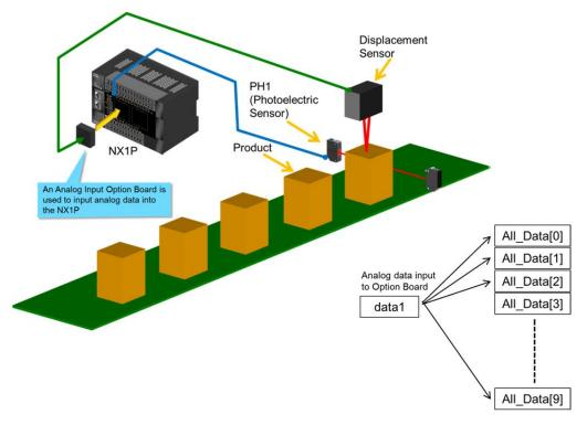
The value measured by the Displacement Sensor is stored in variable *data1* as analog data and then stored as an element of array variable *All\_Data*.
