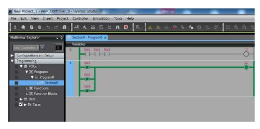
**3.** Double-click the input. You can change the value between True (ON) and False (OFF) to debug the program, instead of pressing the physical switch.
