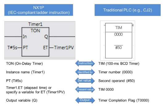
The TON instruction changes timer output Q to TRUE when the set time PT elapses after timer input *In* changes to TRUE.
