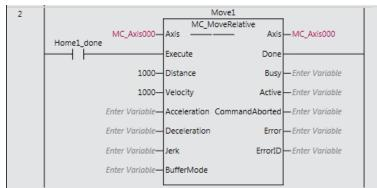
**8.** In the same way as step 6 and 7, insert another MC\_MoveRelative motion FB to move the ball screw backward at the same velocity. Enter "Move2" as the instance name. Set the parameter for *Distance* to -1000 to move backward.
