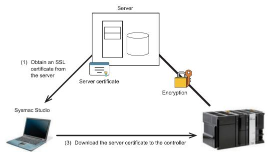
(2) Enable encryption in the Connection Settings Select an SSL certificate (4) Execute a DB Connection Instruction
