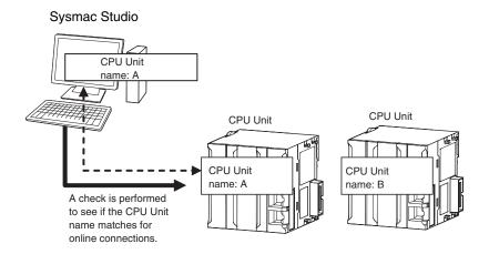
In addition to the CPU Unit name, it is also possible to use serial ID identification based on the CPU Unit production information (optional).
