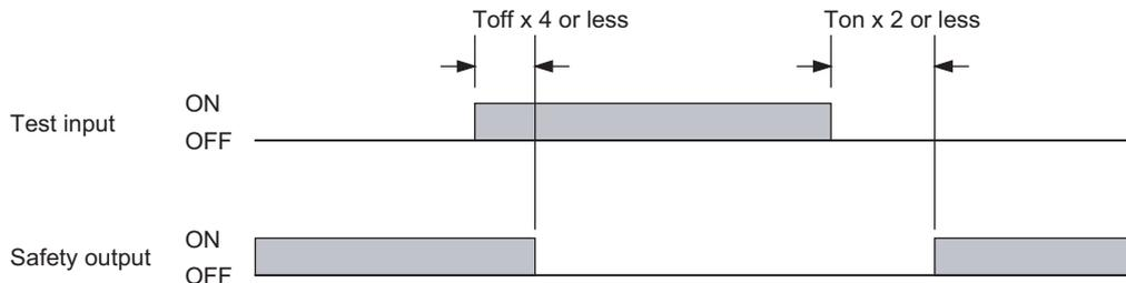
Ton: Response time of safety output's OFF to ON, Toff: Response time of safety output's ON to OFF
