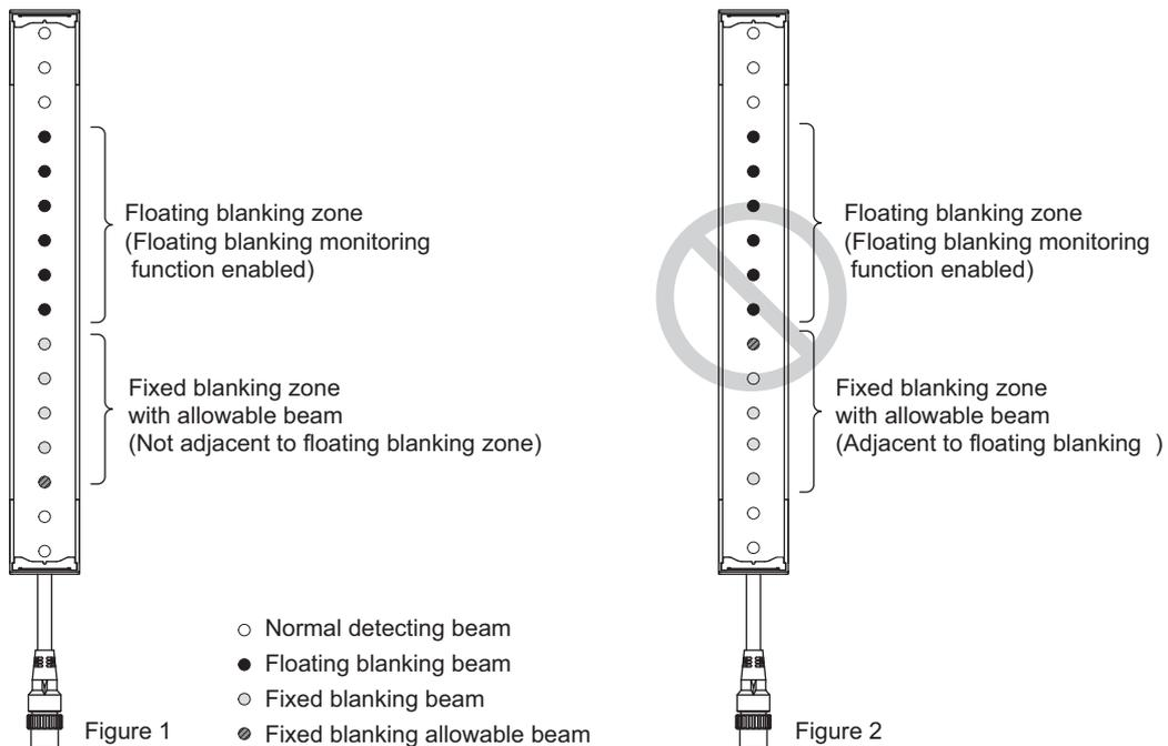
\*2 For details about setting adjacent fixed blanking zones, see the section on fixed blanking.
