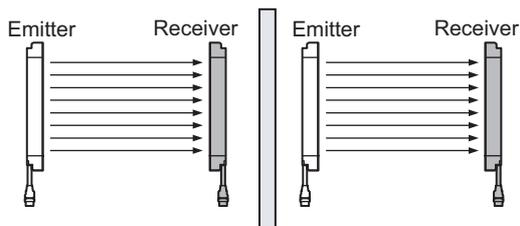
2. Alternate the direction of emission between 2 sets (alternation)
