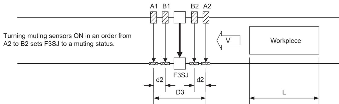
This arrangement example uses regressive reflection type E3Z-R□□ series as a muting sensor. Arrangement must take mutual interference into account.
