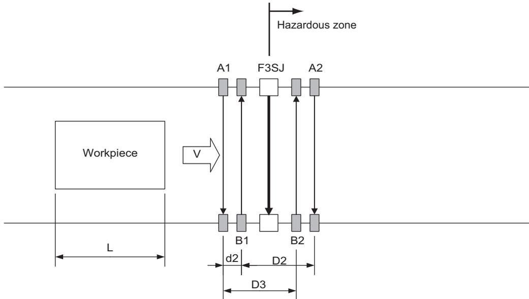
$d2$ : Maximum distance required for the muting sensor to keep the muting function enabled
