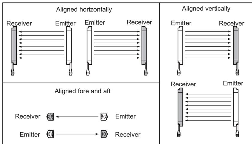
If 2 sets are installed near each other, reflection from the surfaces may cause mutual interference. For such a case, it can be improved by reducing operating range through the setting tool (see Step 3).
