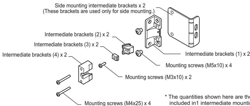
\* The quantities shown here are the number of parts included in 1 intermediate mounting bracket set
