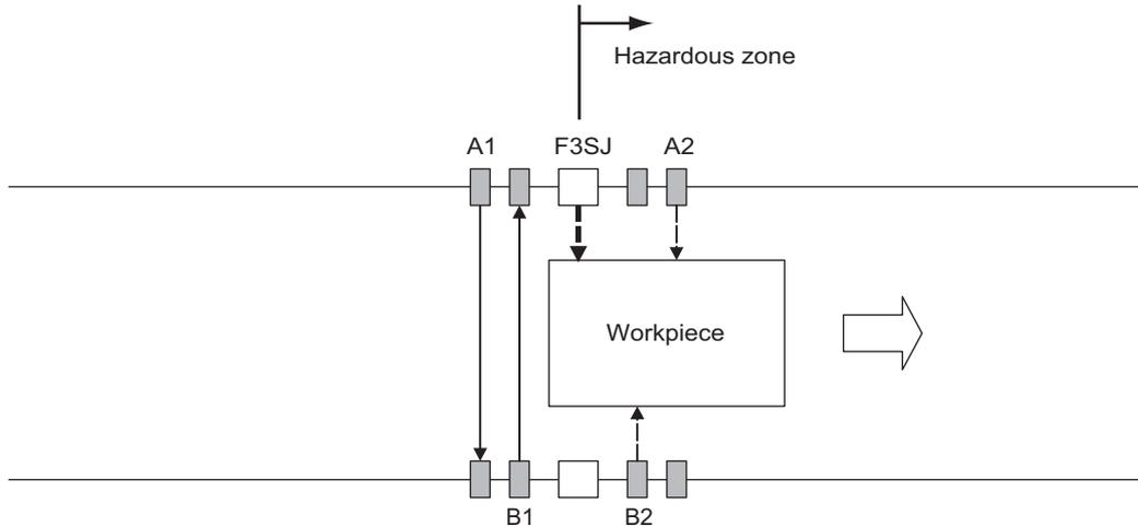
Muting sensors A1 and B1 are turned OFF but A2 and B2 are ON, so the muting function is still working. Safety outputs 1 and 2 are turned ON.
