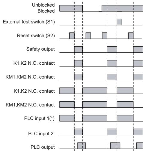
\* Output operation mode of auxiliary output 1 is "safety output information/reverse enabled" (initial setting)
