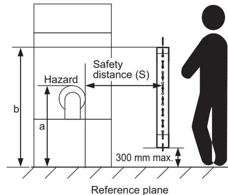
Note: Lower edge of the detection zone above 300 mm in relation to the reference plane does not offer sufficient protection against crawling below.
