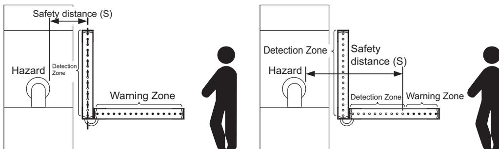
See "Safety Distance: If a person approaches the detection zone of the F3SJ perpendicularly p.111 " if a detection zone is within vertically installed F3SJ as shown left. See "Safety Distance: In case of horizontal approach of a human body to F3SJ's detection zone p.114 " if a detection zone is within horizontally installed F3SJ as shown right.
