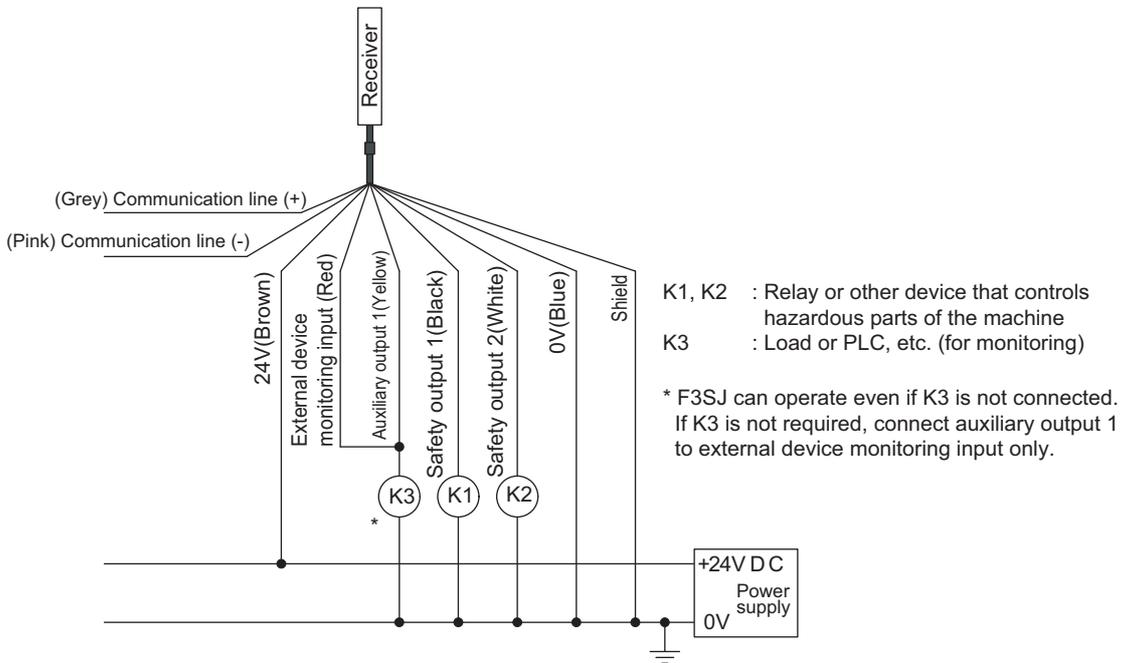
■ Ref.: Minimum Wiring Required to Check the Operation of the F3SJ When Using the Muting Function
