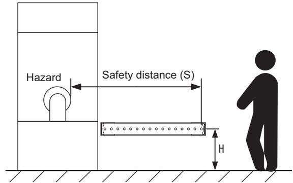
Also, you must include a hazardous condition under which a person may go through under a detection zone carelessly if it exceeds 300mm (200mm for other purpose than industrial use) into risk assessment.
