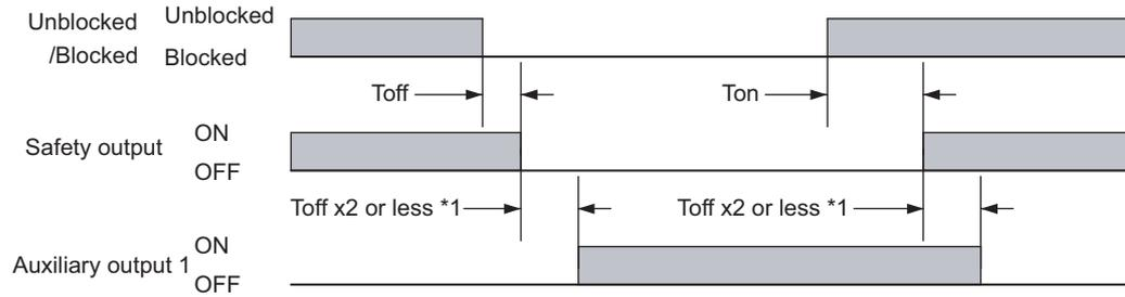
\*1 When a reversed signal of safety output is assigned to the auxiliary output 2 by the setting tool, a delay time of the auxiliary output 2 from the safety output is Toff x 3 or less.
