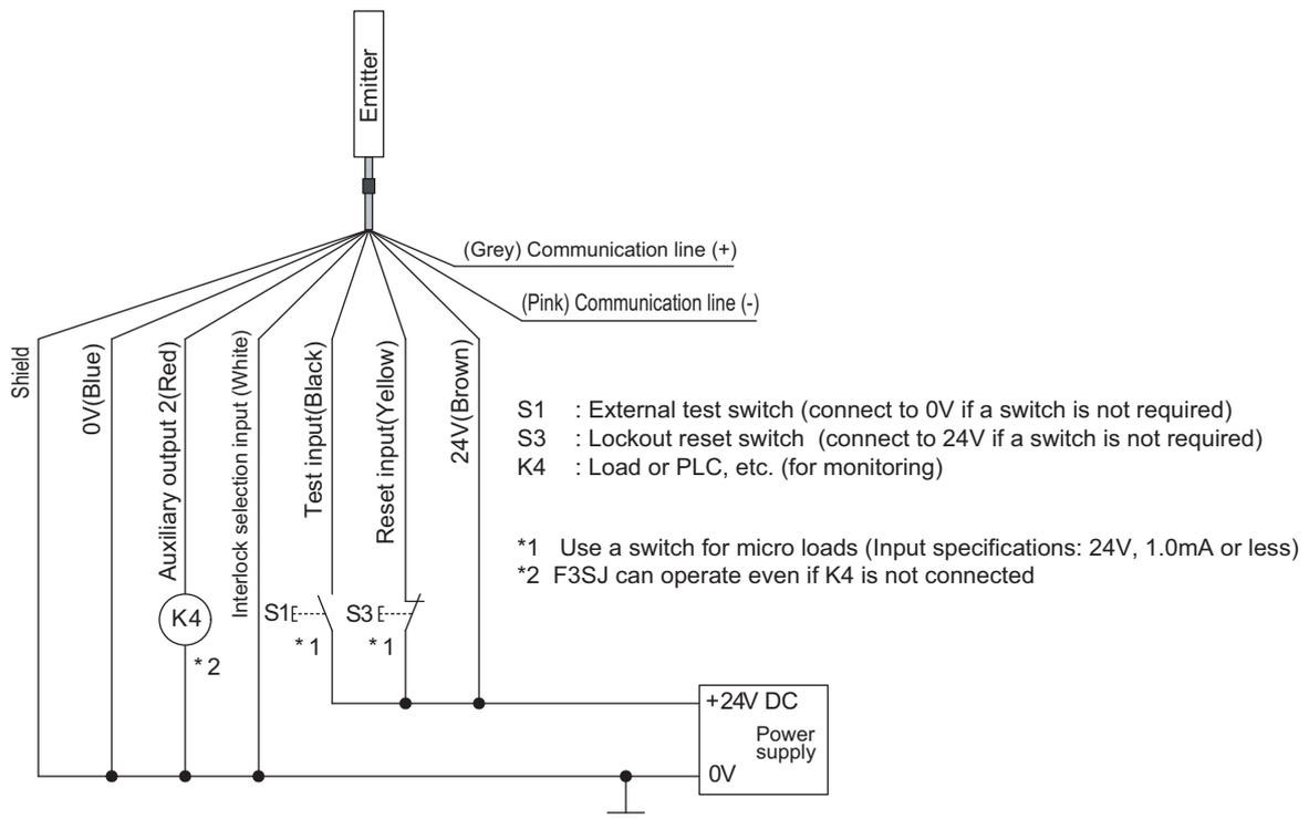
■ Wiring When External Device Monitoring Function Is Not Used
