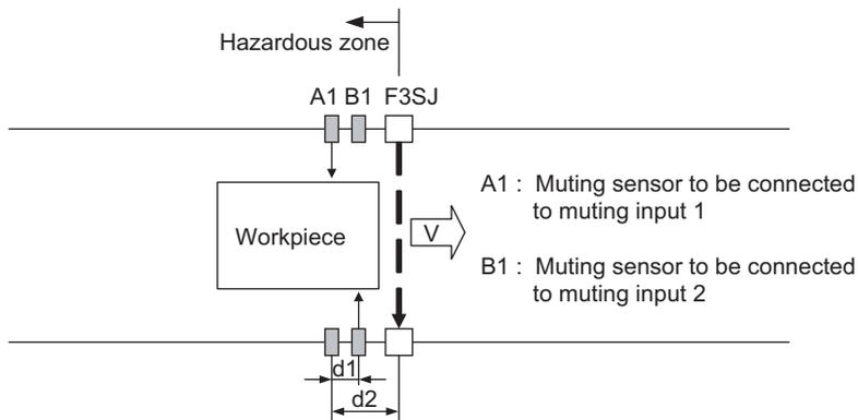
When muting sensors A1 and B1 are turned ON in this order, and the muting function is enabled. In this state, the safety function of F3SJ is disabled.
