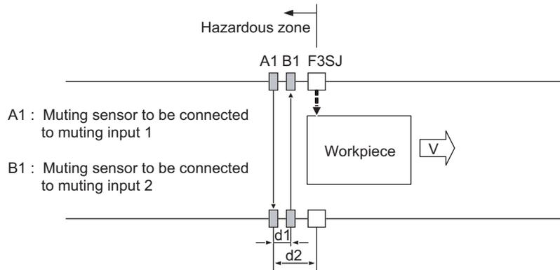
A workpiece finished passing the muting sensor B1 and the sensor is turned OFF. F3SJ disables its safety function if it is within a exit only muting delay time.
