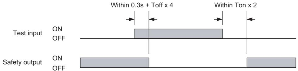
Ton: Response time of safety output's OFF to ON, Toff: Response time of safety output's ON to OFF
