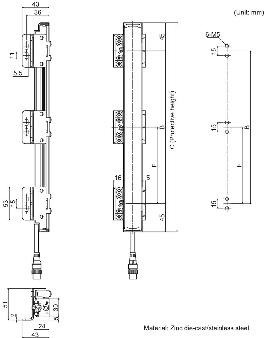
Side mounting (when not using intermediate brackets for side mounting)
