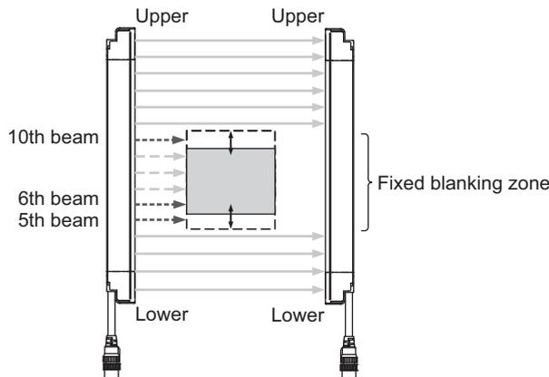
Number of allowable beams available for configuration for each number of fixed blanking beams
