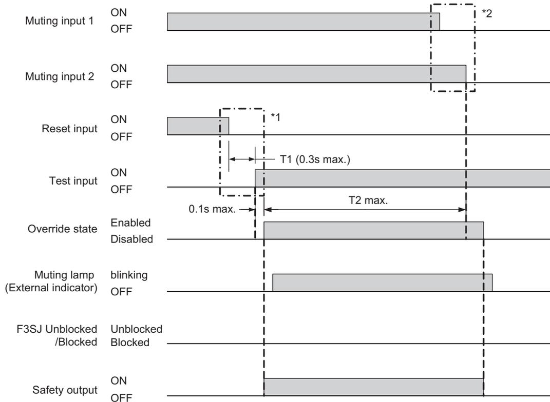
\*1 Order of reset input ON -> OFF and test input OFF -> ON can be arbitrary for override start conditions. (Switching time difference must be within 0.3s)
