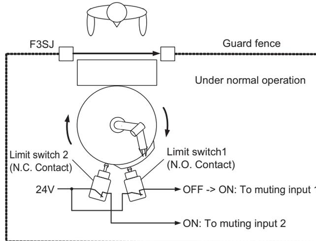
Rotation of a robot arm sets the muting input 1 from OFF to ON. Safety function of F3SJ is enabled.
