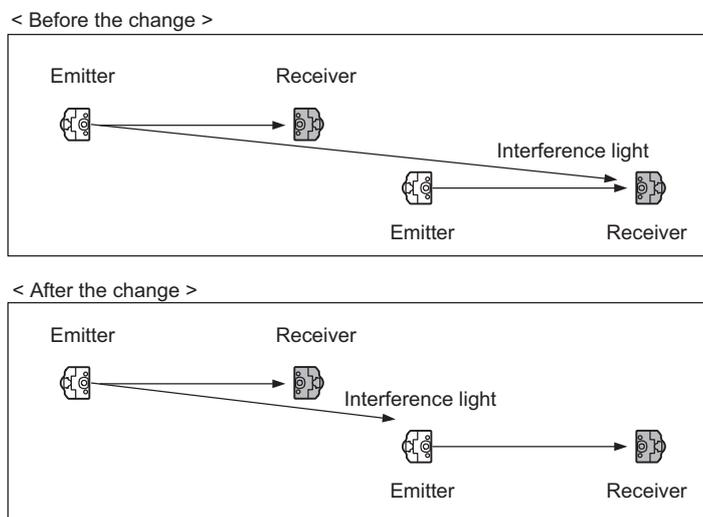
4. Keep sufficient distance between the F3SJs so that mutual interference does not occur
