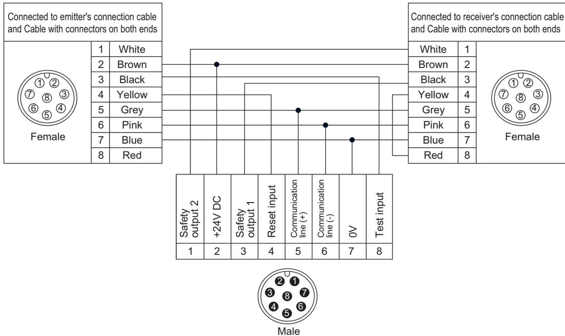
■ Universal indicator cable: A cable for connection with a commercial indicator (optional: F39-JJ3N)
