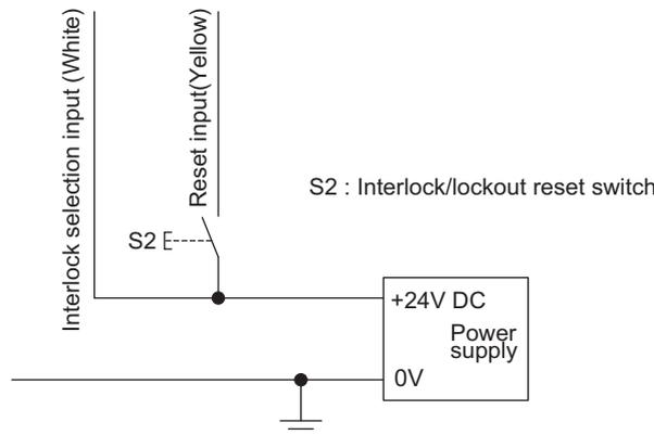
Wiring for manual reset mode p.23
