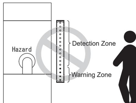
A warning zone must be configured based on a safety distance.
