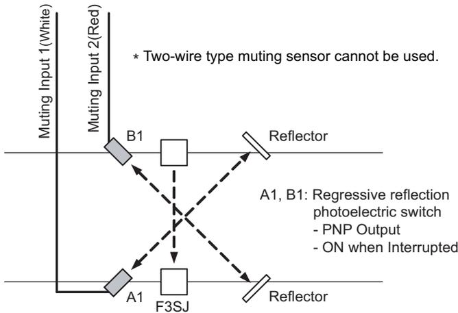
Using an N.O contact type switch as a muting sensor
