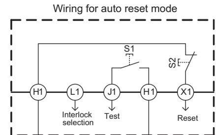
Wiring when not using external device monitoring function
