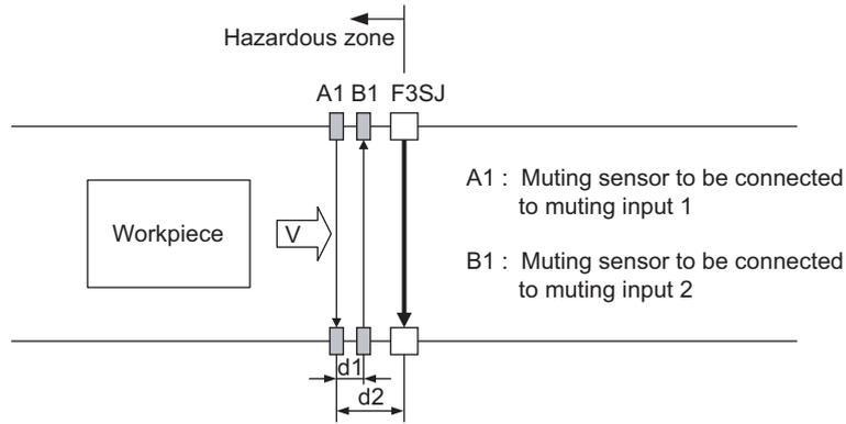
All muting sensors are turned OFF and the safety function of the F3SJ is working.
