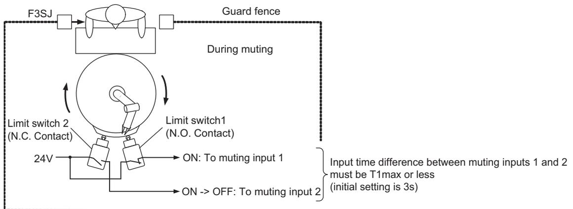
When the muting input 1 turns from OFF to ON and when the muting input 2 is turned from ON to OFF within  $T1_{max}$  [s] before or after the muting input 1's turning ON, safety function of F3SJ is disabled. (Safety output is kept ON even if F3SJ is blocked)
