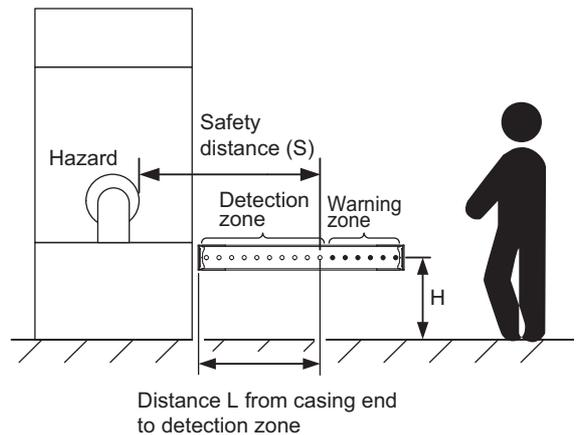
■ How to calculate the safety distance specified by American standard ANSI B11.19 (reference)
