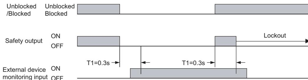
T1: Allowable delay time (can be changed by the setting tool. 0.1 to 2.5s)
