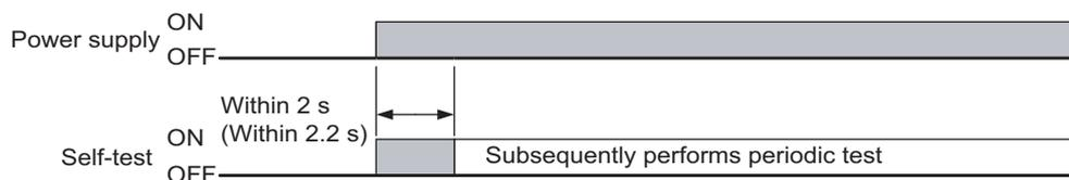
If an error is found in the self-test, the F3SJ enters lockout state, keeps the safety outputs in the OFF state, and indicates the error at the same time.
