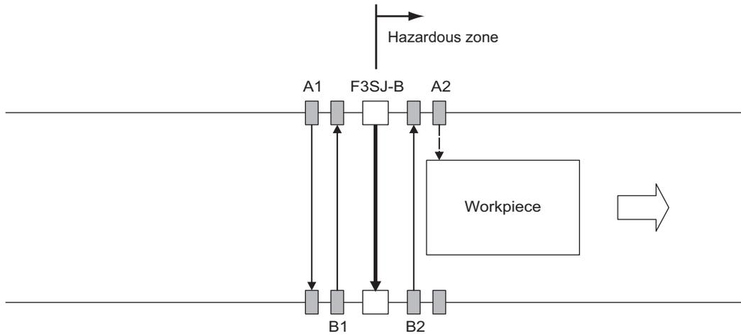
Muting sensor B2 is turned OFF, the muting function is released, and the safety function of the F3SJ-B is enabled.
