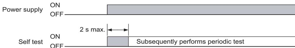
If an error is found in the self-test, the F3SJ-E/B enters lockout state, keeps the safety output in the OFF state, and indicates the error at the same time.
