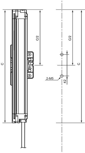
• Mounting with three Intermediate Brackets
