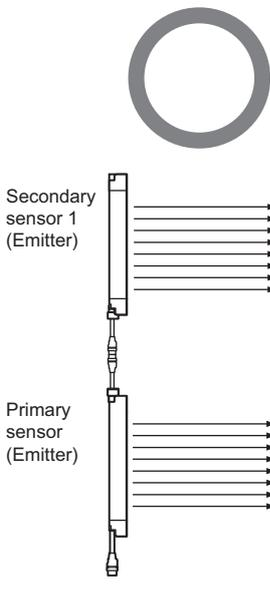
Do not series-connect an emitter and receiver. They will enter lockout state.
