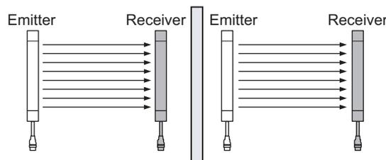
**2.** Alternate the direction of emission between two sets (alternation)
