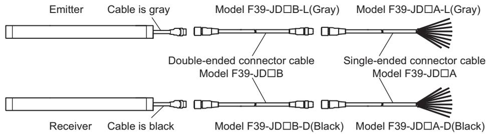
■ Simple Wiring Connector System
