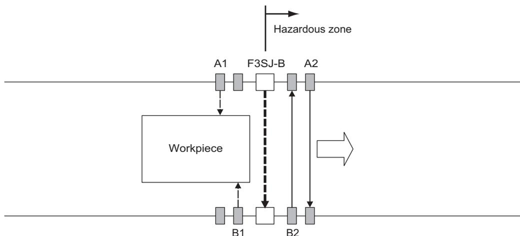
When muting sensors A1 and B1 are turned ON in this order, the muting function is enabled. In this state, the safety function of F3SJ-B is disabled.
