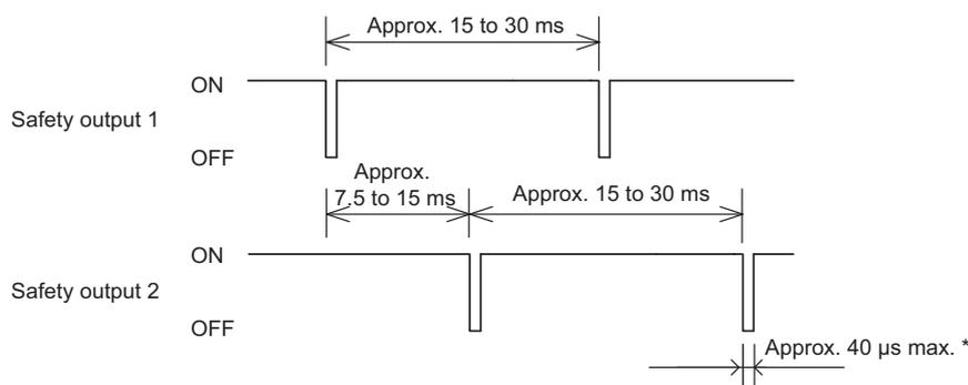
\* An OFF pulse signal of safety output may extend to a maximum of about 100μs due to the effect of the connected load (mostly capacitive load).
