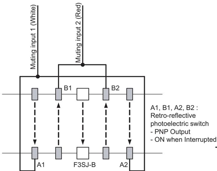
Using an N.O. contact type switch as a muting sensor
