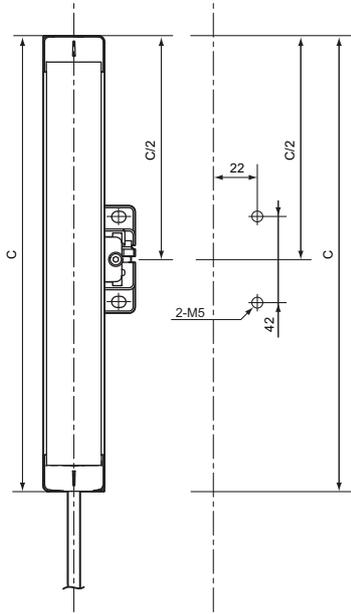
• Mounting with three Intermediate Brackets
