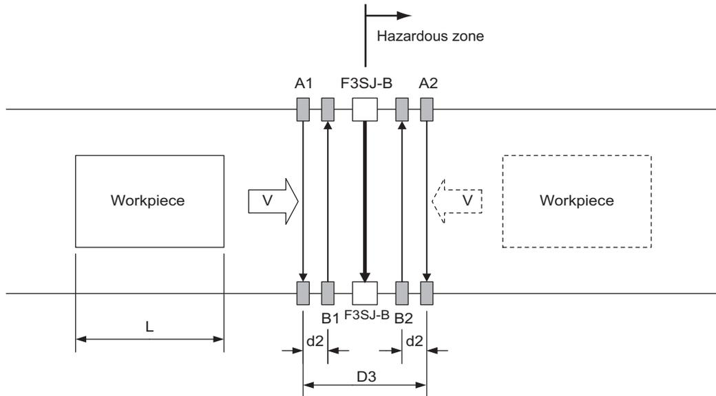
$d2$ : Maximum distances required for the muting sensor to keep the muting function enabled
