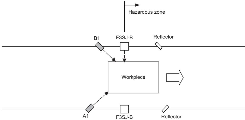
The F3SJ-B is blocked but the safety function is disabled by the muting function, and safety outputs 1 and 2 are turned ON.
