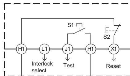
Wiring when not using external device monitoring function
