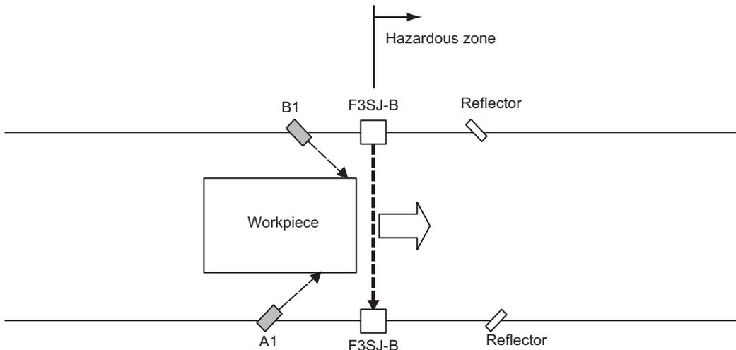
When muting sensors A1 and B1 are turned ON in this order, the muting function is enabled. In this state, the safety function of F3SJ-B is disabled.
