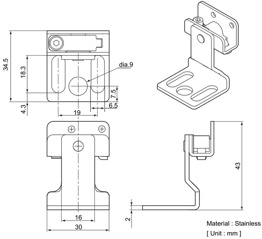
■ Dimensions of Intermediate Brackets (backside mounting)
