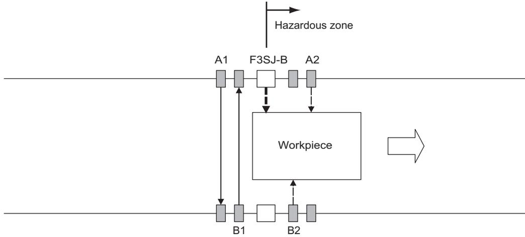
Muting sensors A1 and B1 are turned OFF but A2 and B2 are ON, so the muting function is still working. Safety outputs 1 and 2 are turned ON.
