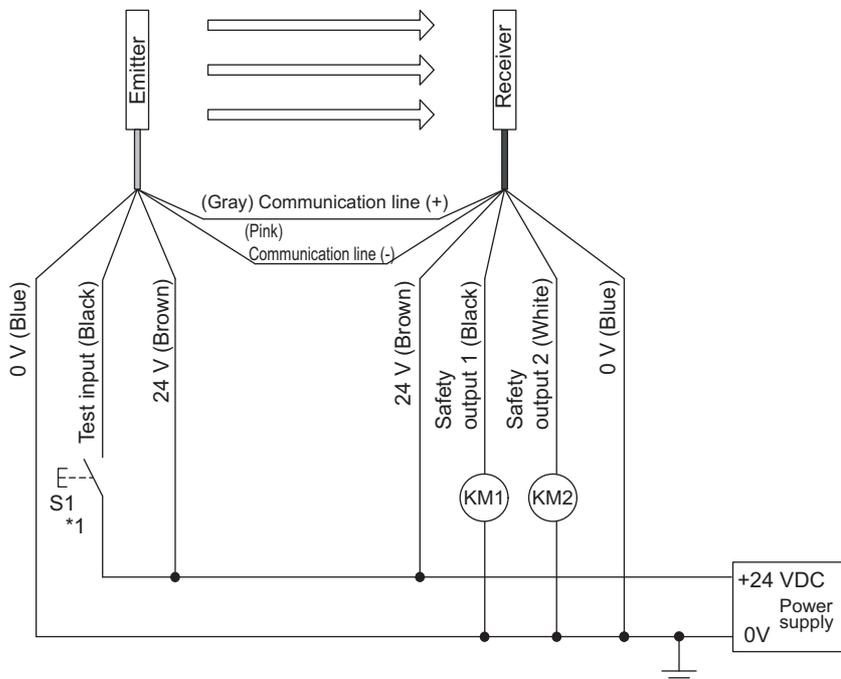
S1 : External test/lockout reset switch (connect to 0 V if a switch is not required)
