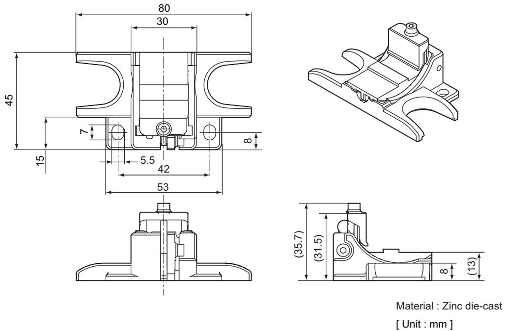
■ Dimensions of Intermediate Brackets (side mounting)
