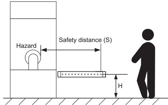
Also, you must include a hazardous condition under which a person may go carelessly through under a detection zone if it exceeds 300 mm (200 mm for other purpose than industrial use) into risk assessment.
