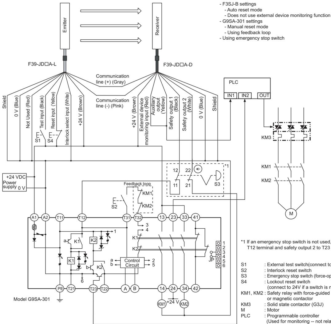
\*1 If an emergency stop switch is not used, connect safety output 1 to T12 terminal and safety output 2 to T23 directly.
