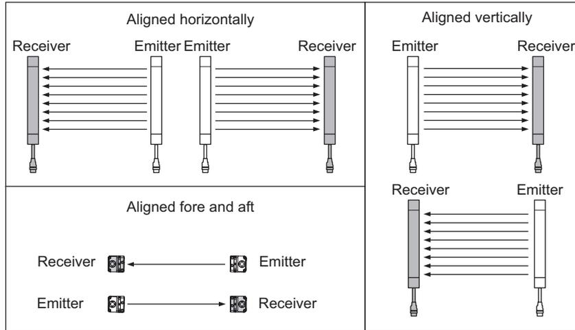
If two sets of F3SJ-E/Bs are installed near each other, reflection from the surfaces may cause mutual interference.
