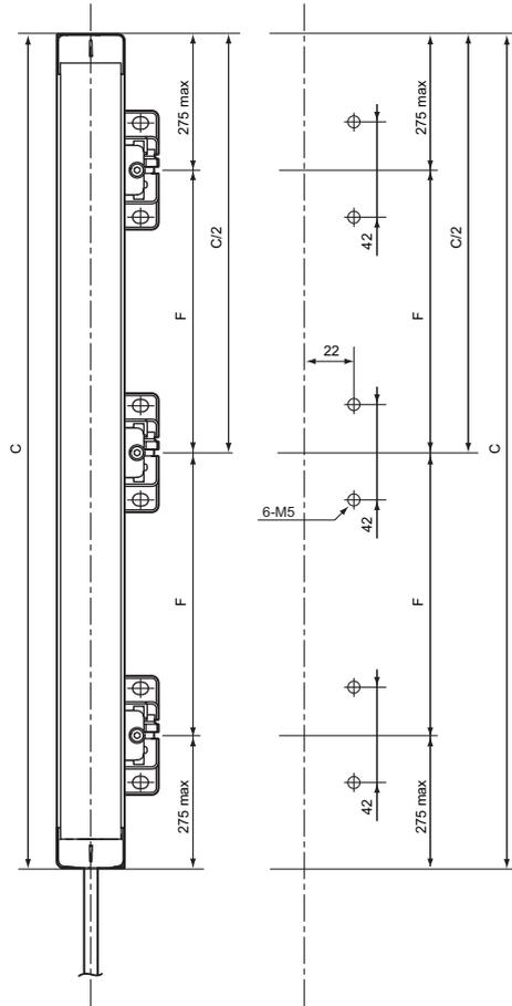
• Mounting with four Intermediate Brackets
