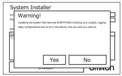
10 When the following message is displayed, remove the media from the NA Unit and turn OFF the power supply to the NA Unit.
