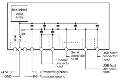
\*1. Protective grounding is not required for the NA5-\(\subseteq\) W\(\subseteq\) \(\subseteq\)-V1-P, and thus no wiring is necessary.
