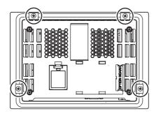
For the NA5-\( \subseteq \text{W} \subseteq \subseteq \text{V1-P}, the locations where the NA Unit must be secured with mounting brackets are the marked locations below.
