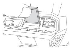
**2** Push the SD Memory Card securely into the compartment.
