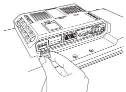
3 Insert the wires all the way to the back of the connector and then turn the screws clockwise to secure the wires.
