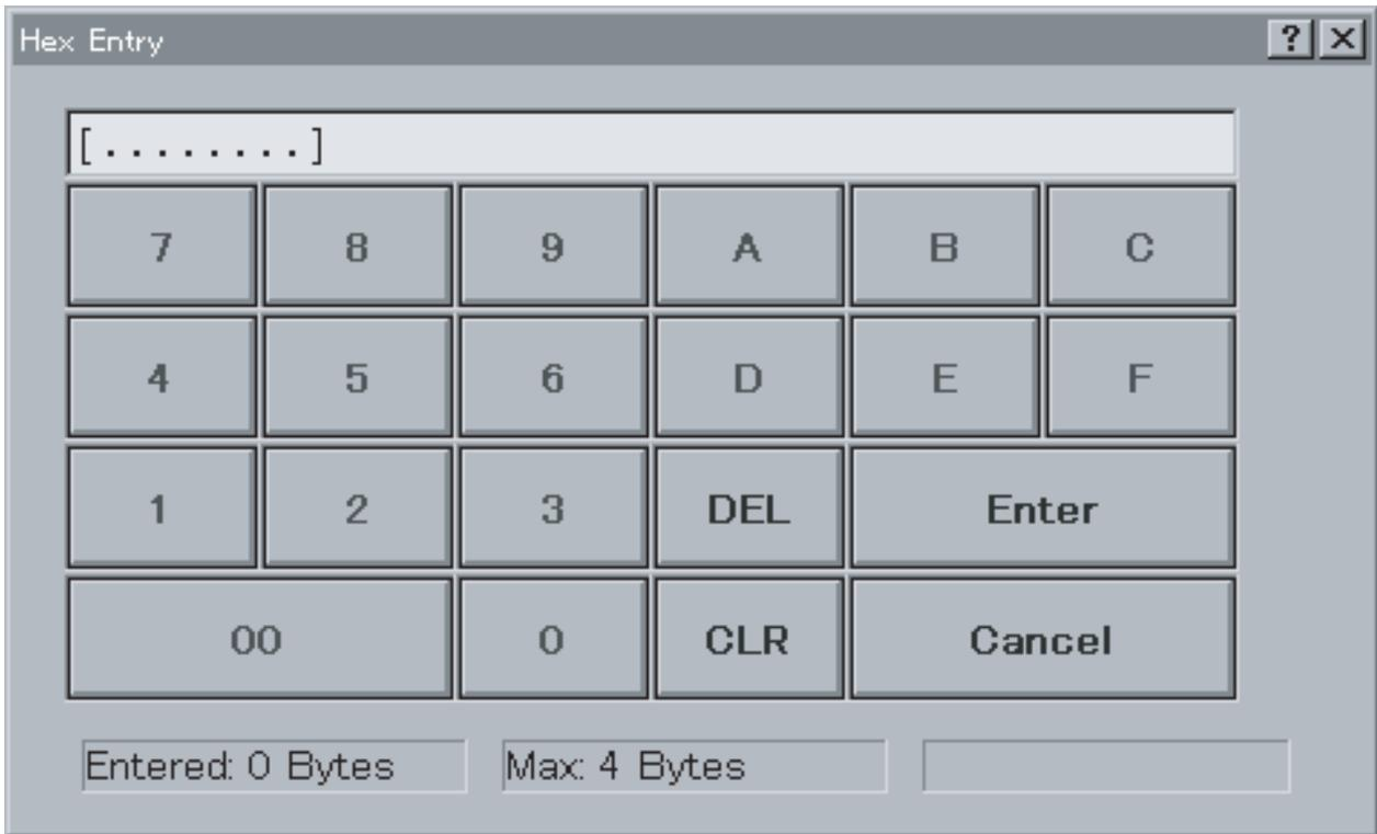
3. Input the required hexadecimal value by left-clicking the button for each digit of that value. Up to eight digits may be entered, and they are displayed at the top of the dialog box. (If a ninth digit is entered, the first digit will be deleted.)
