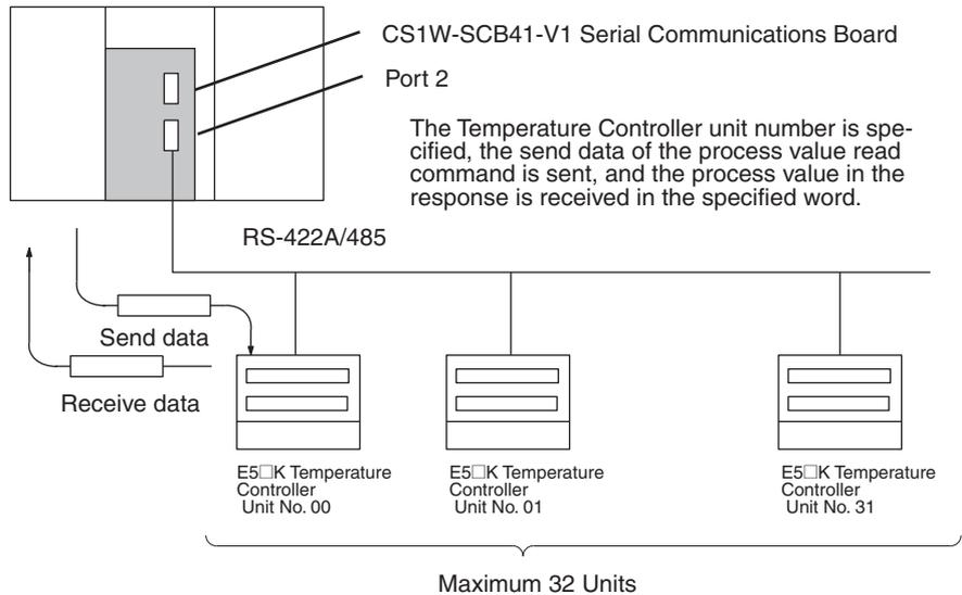
• The Send/Receive Word Allocation Contents of the Sequence No. 000 (read process value)
