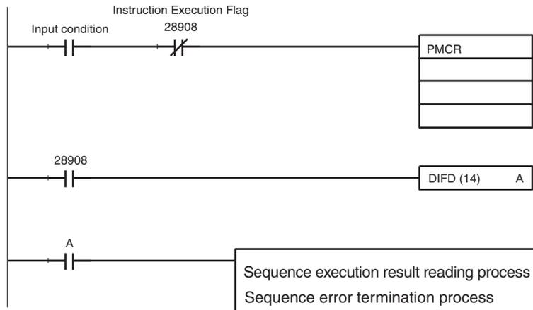
Example: Execution of the protocol name “Controller (E5\_K read)” Sequence No. 000 (“Process value read”)
