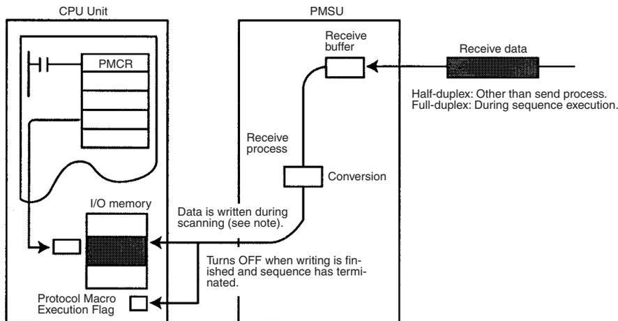
**Note** With the scan notification method, write timing will vary as shown below depending on the PMSU model.
