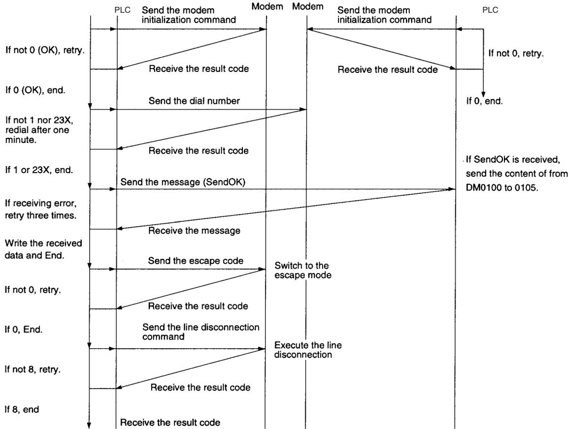
**Note** Information about the AT commands to be sent to the modem i.e. the initialization command, dial command, escape code sending, line disconnection command, etc. and result codes (response) is described in the manual of the modem in use. The modem used in this example is MD24FB10V (made by OMRON). AT commands and result codes supported by the modem are listed in the following tables.
