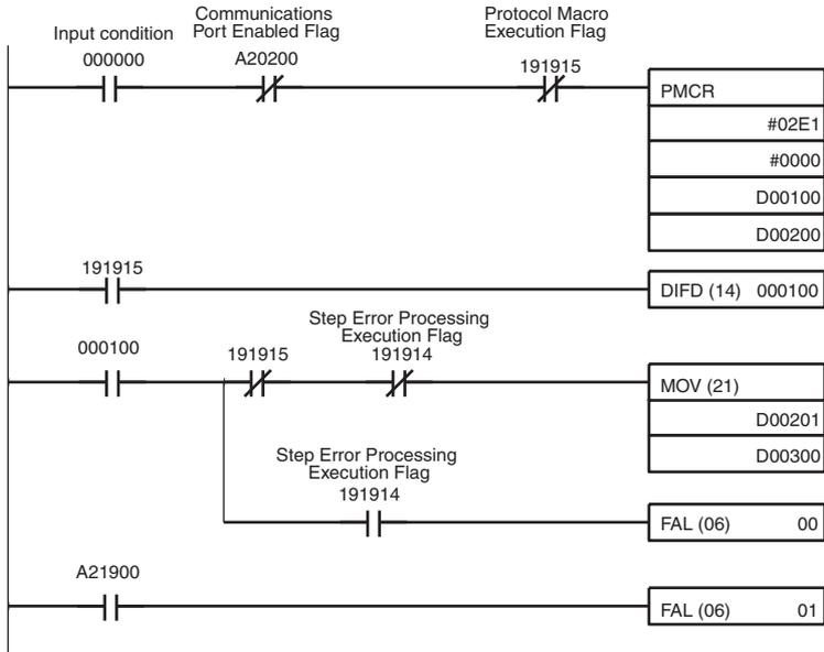
When the input condition 000000 is ON, the Communications Port Enabled Flag A20200 is turned OFF, and the Protocol Macro Execution Flag 191915 is turned OFF, the sequence No. 000 is executed at port 2 of Serial Communications Board, and the process value is stored in D00201.
