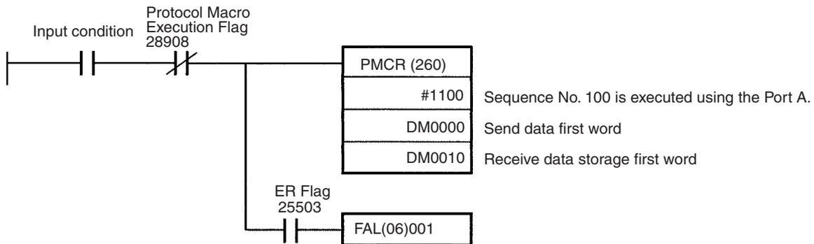
When the input condition is set to “ON” and the Protocol Macro Execution Flag (28908: port A) is set to “OFF,” the communications sequence No. 100 registered on the PMSU will be called to send and receive data via port A of the PMSU.
