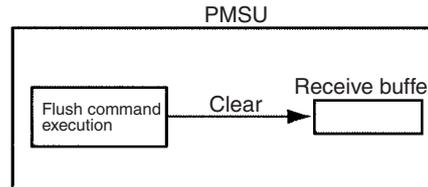
This command can also be used, for example, in full-duplex mode when a communications error occurs. Without aborting, switch the step in Goto, execute the Flush command in the step, clear the receive buffer, and retry.
