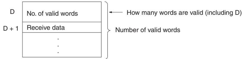
**Note** The function of the receive data storage area (the data stored in the area starting with D and continuing for the number of words indicated in D) before the PMCR instruction is executed, differs to the function of the area afterwards.
