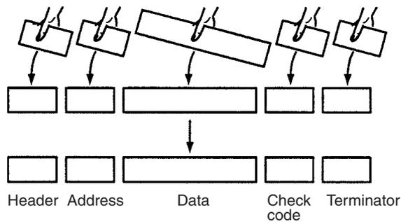
**Note** In general, the data area of a send message contains a command code and data. The data area of a receive message contains a response code.
