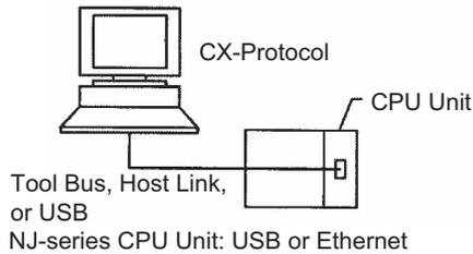
Connecting to PLC through Serial Communications Board or Unit
