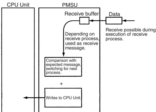
Data received during sending will not be used as receive data. Data received when not sending will be sent to the receive buffer. This data can be extracted using the receive process.
