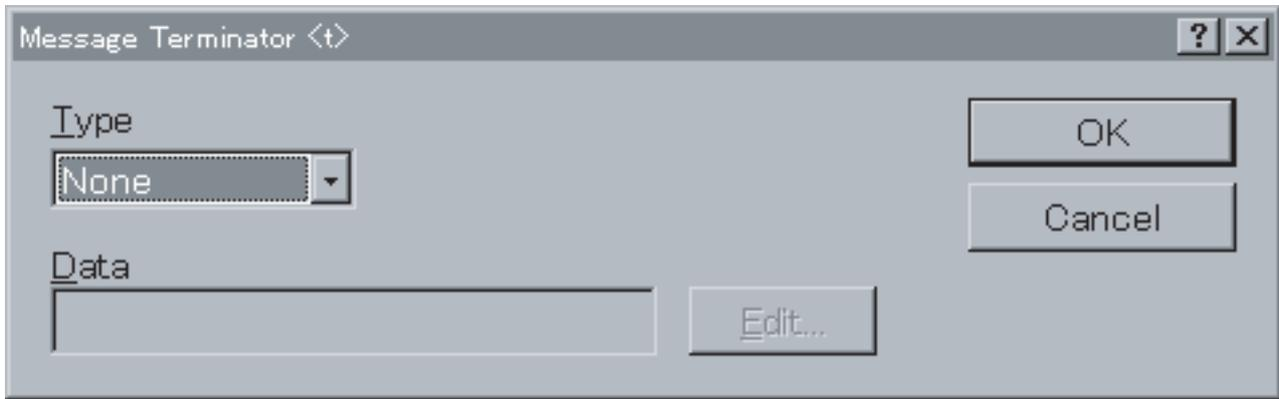
Select a terminator type from the **Type** drop-down list and set the **Data** Field. (For inputting the Code, ASCII, or Hexadecimal, refer to the previous *Header <h>* section.)
