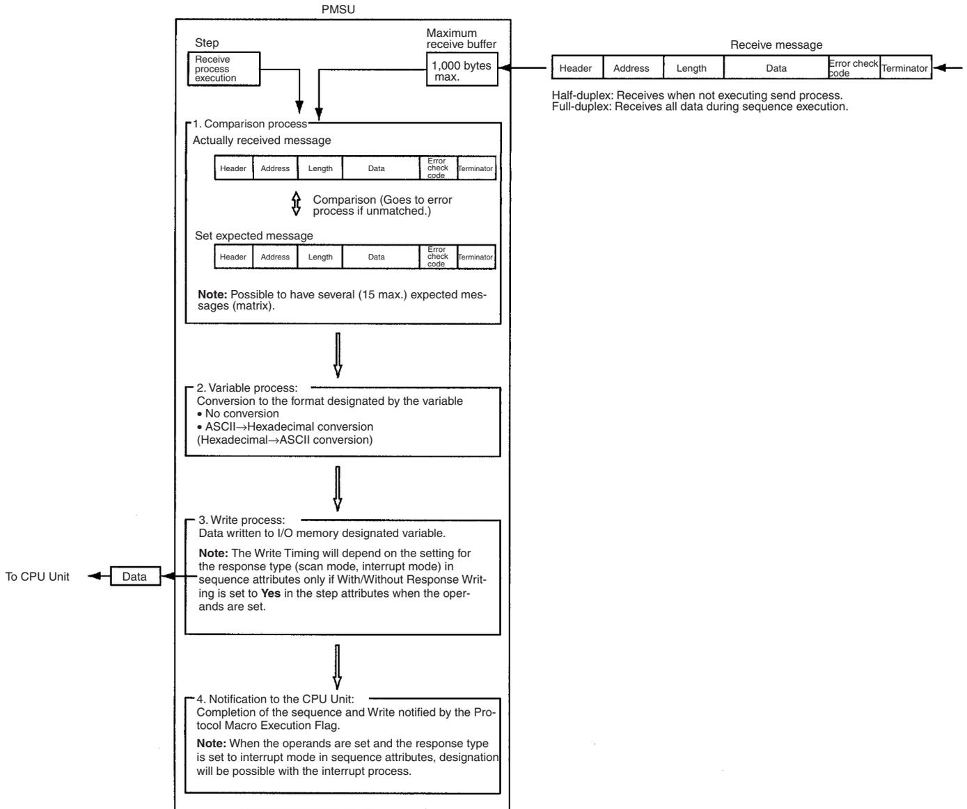
**Send & Receive Process (Send & Receive Command)**
