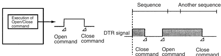
When the transmission control parameter is set to modem control for the conventional protocol macro for the C200HX/HG/HE, the DTR signal will turn ON when a sequence is started and will turn OFF when sequence execution is completed. This setting has the following problems.
