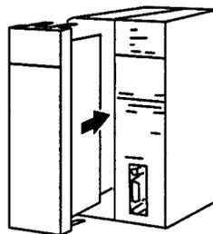
Mounting the Serial Communications Unit
