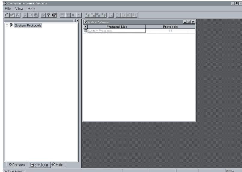
The CX-Protocol can be started also by right-clicking a Serial Communications Board/Unit in the I/O Table Window opened from the CX-Programmer and selecting **Start Special Application** from the pop-up menu.
