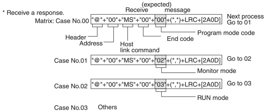
By using the matrix, identify the difference in the status in the response data (section in the above), and change over the process according to the mode of the PLC.
