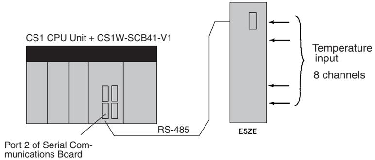
Eight points of measured temperature are stored in DM 00101 to DM 00116.
