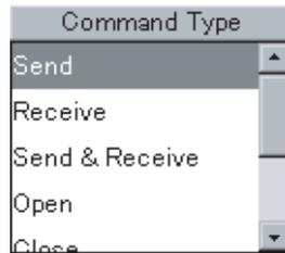
**Note** When set to modem control mode, the DTR signal will turn ON when the sequence is started and will turn OFF when the sequence ends. If the DTR signal is turned ON using the Open command under the modem control mode, the DTR signal will remain ON even after the sequence has ended.
