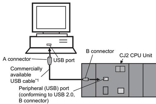
\*1 Commercially available USB cable: 5 m max., for USB 1.1 or 2.0.
