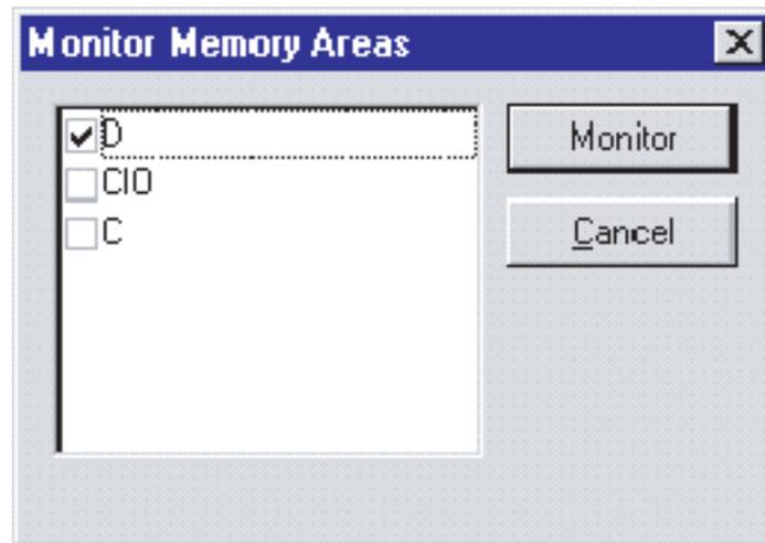
4. Select the area to be monitored and left-click the **Monitor** Button. The displayed range of the selected area in the PLC data window will be monitored.
