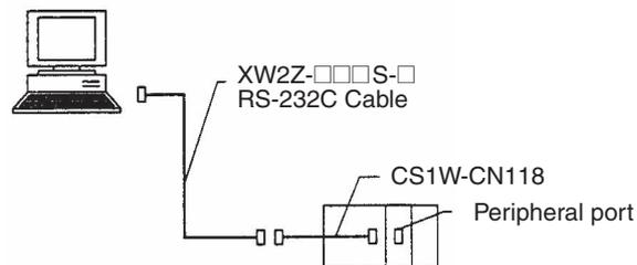
When combining the CS1W-CN118 with the RS-232C Cable, connections cannot be made using the **Toolbus**. Make connections using **Host Link (SYSWAY)**.
