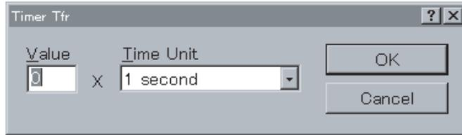
2. For receive wait time (Tr), set in the **Value** Field a monitor time (0 to 99) from recognition of a receive command to reception of the first byte of data. For receive finish time (Tfr), set in the **Value** Field a monitor time (0 to 99) from reception of the first byte of the data to the last byte of the data. For send finish time (Tfs), set in the **Value** Field a monitor time (0 to 99) from the transmission of the first byte of the data to the last byte of the data.
