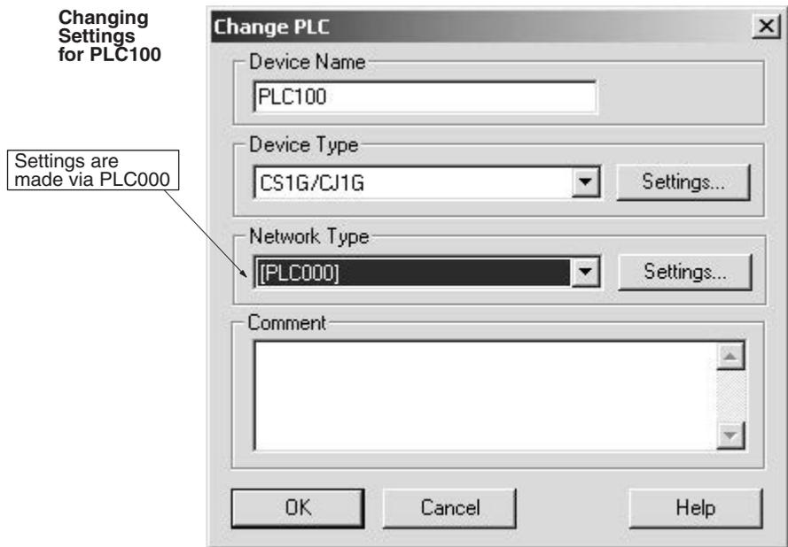
By making the above settings, PLC000 becomes the gateway for communications with PLC100. To make an online connection, right-click **PLC100** in the project workspace and select **Connect to PLC**, or select **Connect to PLC** from the **PLC** Menu.
