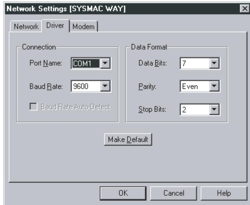
Note The communications conditions must coincide with those in the PLC Setup of the CPU Unit. For details, refer to the Operation Manual of the PLC.
