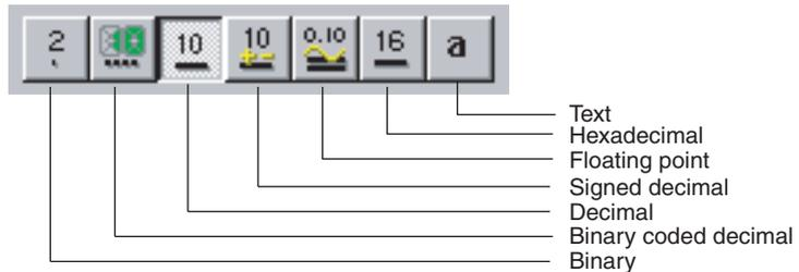
**Note** The default data display format in the PLC data table can be changed by selecting the new default data display format from the **Display** Tab in **Preferences** in the **Display** Menu.
