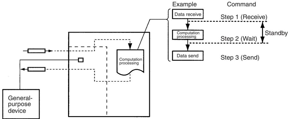
If used in combination with a matrix, it is possible to set up the system so that when certain data is received, the send/receive sequence will be put on standby and computational processing (e.g. data processing) will be performed at the CPU Unit before proceeding to the next communications process.
