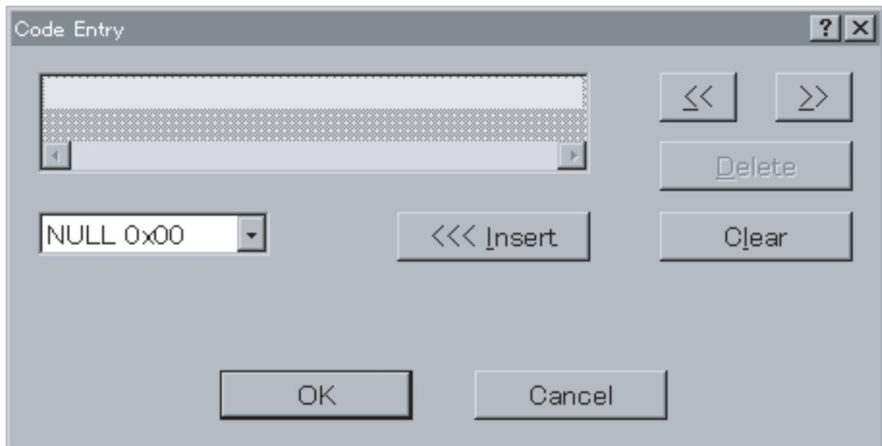
3. Select **Special Code**. Up to four special codes may be entered. Select the codes from the drop-down list and left-click the **Insert** Button to input the code indicated.
