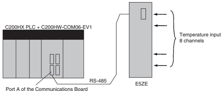
Eight points of measured temperature are assumed to be stored to DM101 to DM 116.
