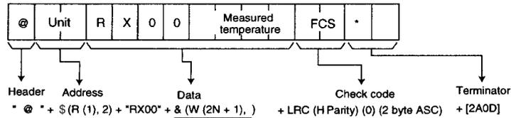
Means that the system reads the data between RX00 and the check code, converts the data from ASCII to Hex, and writes the converted data to the address of the fourth (third for C200HX/HG/HE) operand of the PMCR instruction + (2N+1)
