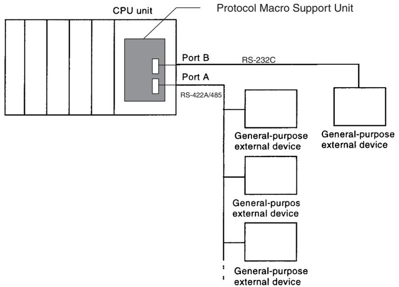
**Note** For connector pin arrangements and connection methods, refer to the *Communications Board Operation Manual (W304)* and other relevant manuals for general-purpose external devices.
