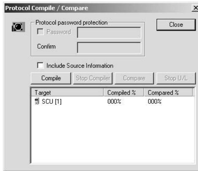
5. If the source code was also transferred with the protocols the last time the protocols were transferred to the Board/Unit, select the *Include Source Information* Option.
