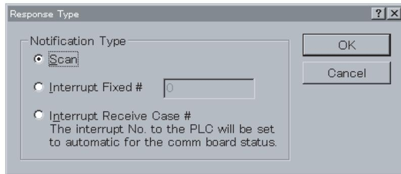
2. Select one of the notification types: **Scan**, **Interrupt mode: Fixed #** or **Interrupt mode: Receive Case #**. When the **Interrupt mode: Fixed #** Button is left-clicked, designate the external interrupt task number for the CS/CJ or the interrupt subroutine number for the C200HX/HG/HE in a range from 0 to 255.
