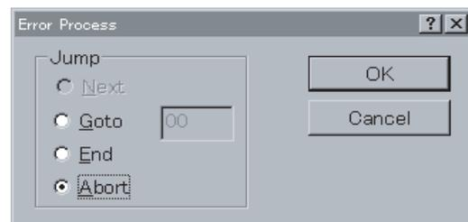
When one of the following error factors occurs, the step ends abnormally, and then the system goes to the appropriate error process.
