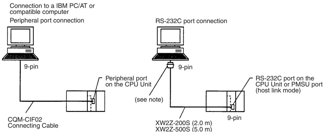
**Note** For IBM PC/AT or compatible computers, a conversion connector from D-sub 25P (female) to 9P (female) is required for the personal computer side connector.
