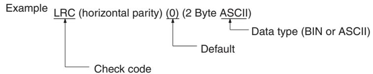
Note Set the calculation range of the error check code <c> in the **Data** Field of the **Message Editor** Dialog Box.
