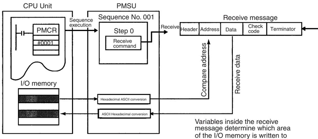
To designate which area of I/O memory is used for creating send messages and which area of I/O memory is used for storing receive messages, the following three methods can be used.
