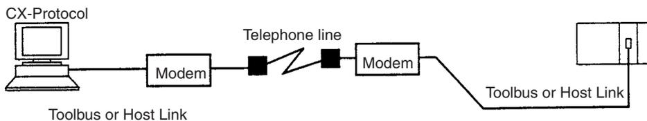
**Note** This type of connection is not supported for an NJ-series CPU Unit.
