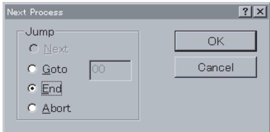
2. Select Next Process from the **Jump** Field. When **Goto** is selected, input a step number in the empty field.
