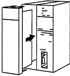
Mounting the Serial Communications Unit on the CPU Rack
