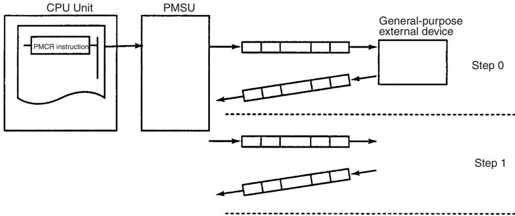
2. This step can be set so that the next process (step/end) depends on the processing result of the previous step. In particular, it is possible to set the sequence so that the next process depends on the contents of one or several set receive messages.
