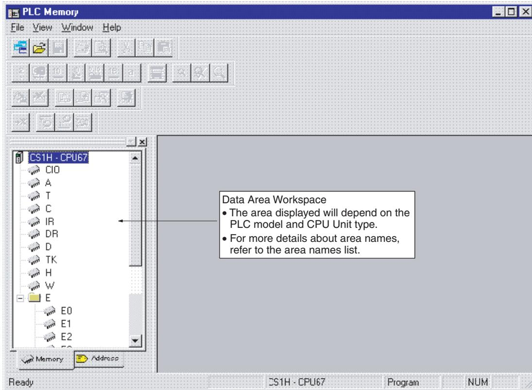
2. Double-click the name of the desired area in the data area workspace. The PLC data table will be displayed. The following example is the PLC data table of the CIO area of the CS/CJ Series.
