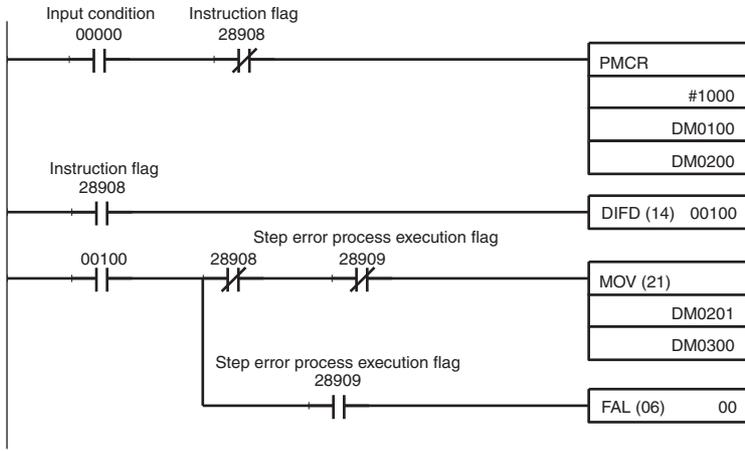
When the input condition 00000 is ON and the Instruction Execution Flag 28908 is OFF, the sequence No. 000 is executed and the process value is stored in DM 0201.
