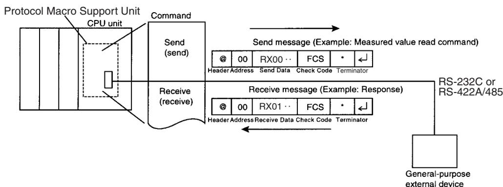
The sequence determines, according to the result of process, whether to send the same send message again (called retry) or execute the next process (reading process value from the Temperature Controller linked to another address, etc.), for example.
