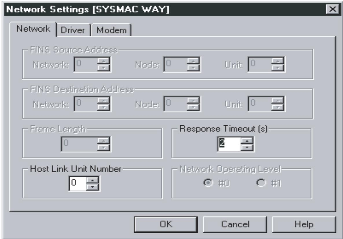
3. Left-click the **Driver** Tab in order to change the communications conditions. The name of port, baud rate, data length, parity, and number of stop bits can be set.
