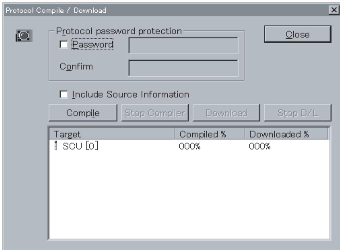
5. Prior to download, a password can be applied to protect the protocol. Select the **Protocol password protection** check box to enable password protection. Enter a password in the **Password** Field (up to eight characters). Enter the password in the **Confirm** Field.
