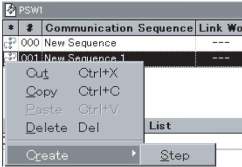
A new step is created after clicking the right mouse button or pressing the **Shift+F10** Keys to select the corresponding item in the popup menu. In this example, **Create/Step** is selected.
