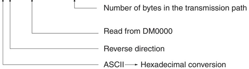
Users can set the following contents on the X and Y of variable (X,Y).
