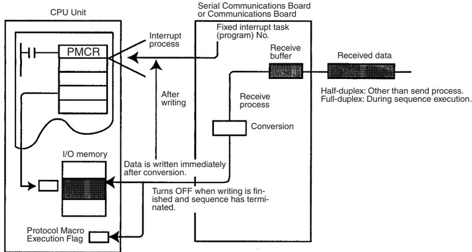
**Note** With the CS-series (Serial Communications Board), received data cannot be stored in the EM area using the interrupt notification. If this is attempted, a protocol macro syntax error (A42410) will occur.
