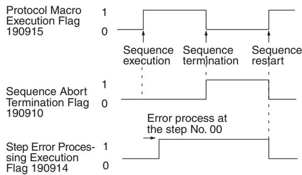
**Note** 1. The Step Error Processing Execution Flag is not a flag for the whole sequence, but a flag to determine whether the error process is executed at a step in the sequence. Therefore, as in the above example 2, if the consec-
