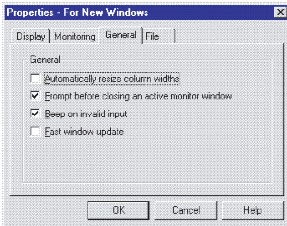
**Automatically resize column widths:** The column widths will be automatically adjusted according to the window size of the PLC data table.
