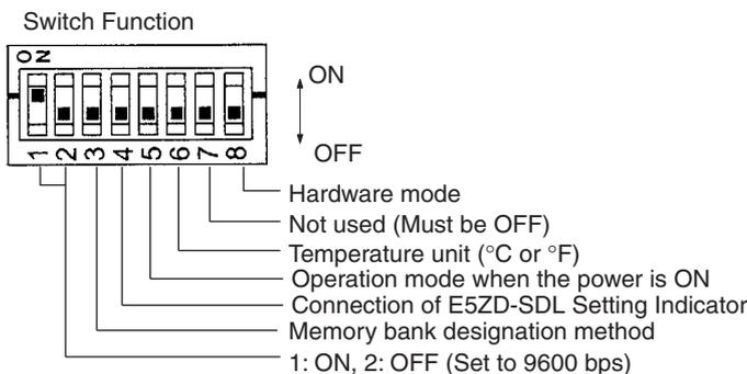
Note After changing the DIP switch's setting, turn OFF and ON the power supply once.
