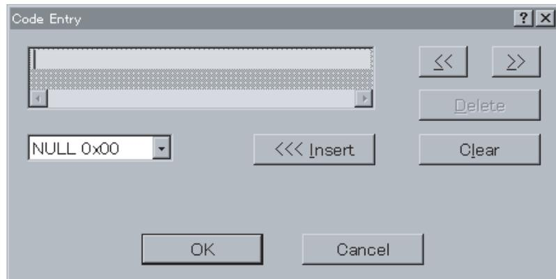
3. Select **Special Code**. Up to four special codes may be entered. Select the codes from the drop-down list and left-click the **Insert** Button to input the code(s) indicated.
