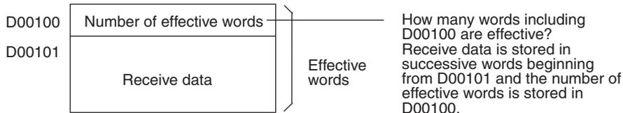
Note Receive data set before the PMCR is executed will not change if receive processing fails.
