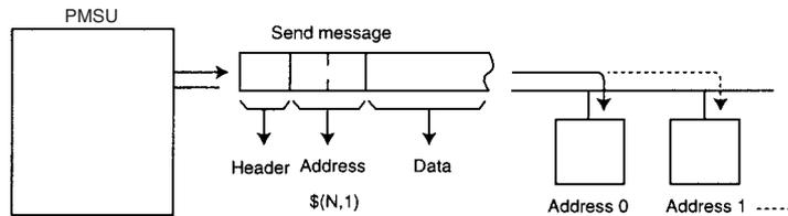
**Example:** If different addresses for different steps are to be designated to store receive messages, include the repeat counter variable N in the data in the receive message.
