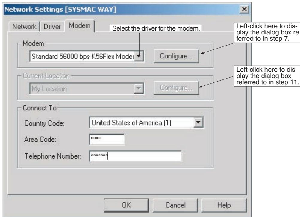
Use the following procedure to make settings for the modem and the present address.
