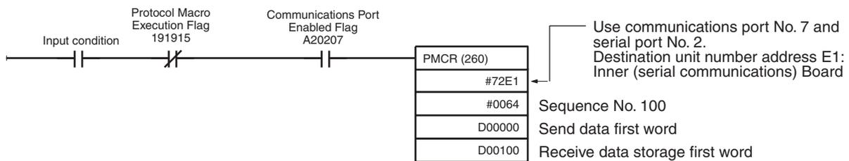
When the input condition is set to “ON” and the Protocol Macro Execution Flag (191915: port 2) is set to “OFF,” the communications sequence number 100 registered on the PMSU is called to send and receive data via port 2 of the PMSU if the Communications Port Enabled Flag (A20207: internal logic port of the communications port No. 7 is used) is ON.
