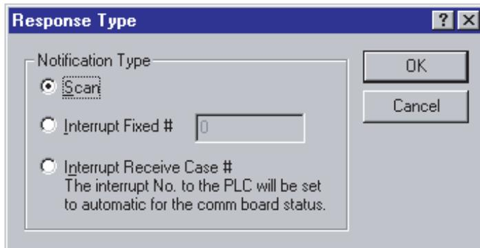
**Note** When an interrupt notification is used with the CS-series (Serial Communications Board), the protocol macro status area (within the interrupt data area) will not be updated completely when the interrupt notification is received. Therefore, read the receive data only after the external interrupt task conditions have been satisfied in order to ensure concurrent data processing. The PMCR instruction cannot be executed within the external interrupt task
