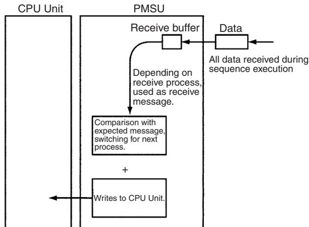
All data received during sequence execution (including data received when not executing the receive process) will be used as the receive message.
