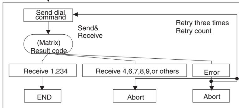
When configuring the steps, the enough consideration is necessary not only for the normal course (the process is completed in normal) but for the error course (the process is terminated by error). The error courses are often set to be aborted (intermittent process stop) all together. However, if the abort is set as the simple "other than normal course," the process stops there.
