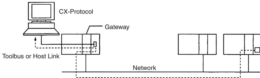
**Note** This type of connection is not supported for an NJ-series CPU Unit.
