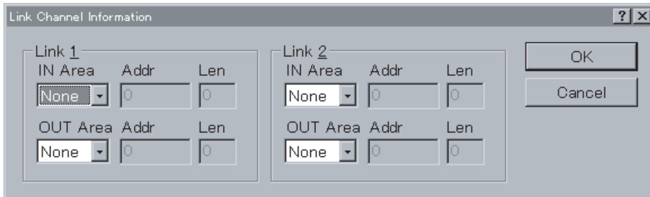
Perform Link 1 setting according to the following procedure. Follow the same procedure for the Link 2.
