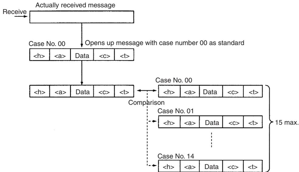
Therefore, if there are differences in message formats between cases because messages are opened up using the frame configuration of case number 00, comparison results for frames with a different message format from case number 00 will register a non-match, irrespective of the actually received message.
