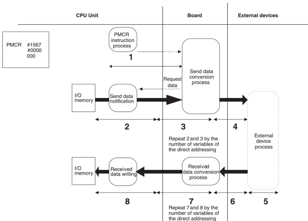
The communications response time is the total time from 1 to 8 in the above figure. The functions 2 and 3 are repeated by the number of variables of the direct addressing of the send message while 7 and 8 are repeated by those of the receive message.
