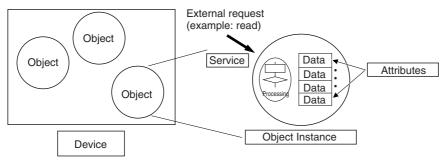
In the CIP Common Specification, "Object," "Class," "Instance," "Attribute," and "Service" are defined as follows: (Source: CIP Common Specification)
