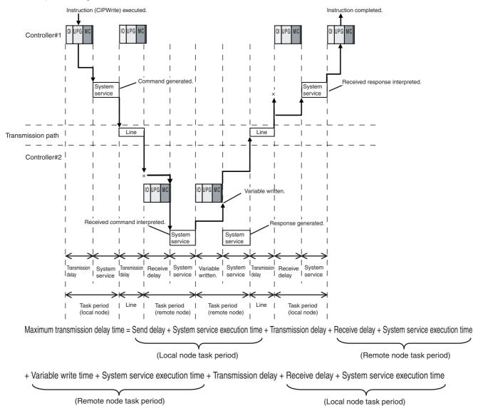
Processes that cause a delay time are processed in the task periods at each node as shown in the above diagram. Line-based delays are as follows:
