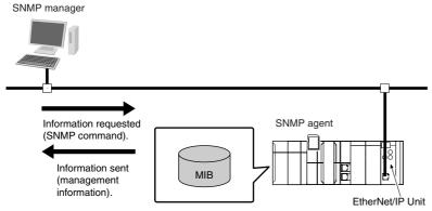
The SNMP manager has a SNMP command to request MIB information. The EtherNet/IP Unit SNMP agent function supports SNMPv1 (RFC1157) and SNMPv2C (RFC1901). Use the SNMPv1 or SNMPv2C protocol to manage the EtherNet/IP Unit with the SNMP manager. You can also use both the SNMPv1 and SNMPv2C protocols together at the same time.
