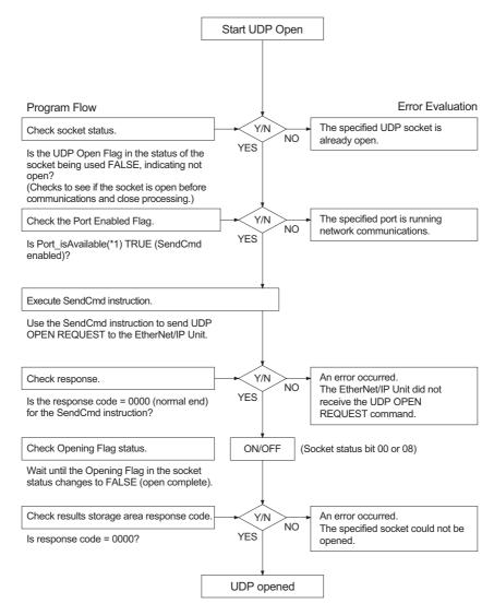
(\*1) \_Port\_isAvailable is a system-defined variable for the Controller to determine whether or not SendCmd is enabled. Refer to the NJ/NX-series CPU Unit Software User's Manual (Cat. No. W501) for details.
