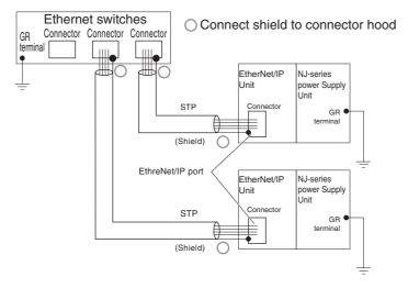
b) Connecting the shields on the Ethernet switch side only
