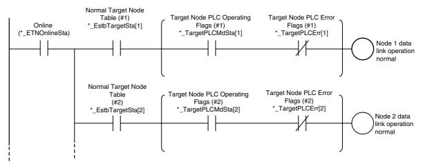
Programming Example 2 to Detect Normal Operation
