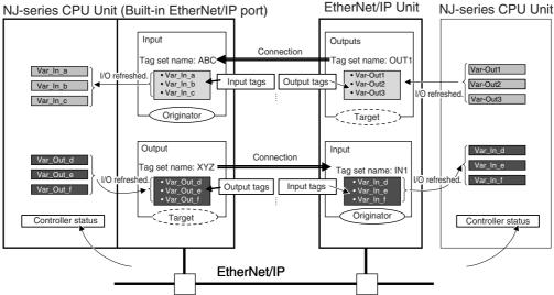
For communications between Controllers, the connection information is set in the EtherNet/IP Unit of the Controller that receives (consumes) the data (i.e., the originator).
