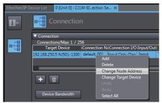
**2** The Node Address Change Dialog Box is displayed. Enter a new IP address in *New IP address*.
