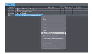
The I/O ports in the source replacement model CJ1W-EIP21 are expanded.
