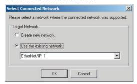
The Network Configurator will connect to the EtherNet/IP network. If the Network Configurator goes online normally, "Online" is displayed in the status bar at the bottom of the window. The network connection icon is displayed in blue on the Network Tab Page in which the Network Configurator is connected.
