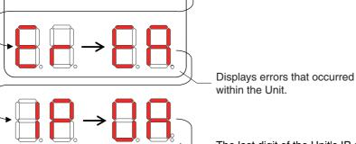
The last digit of the Unit's IP address is displayed in hexadecimal.
