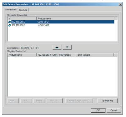
In the Unregister Device List, click the target device that requires connection settings so its color changes to gray, and click the Button. The selected target device is displayed in the Register Device List, as shown in the following diagram.
