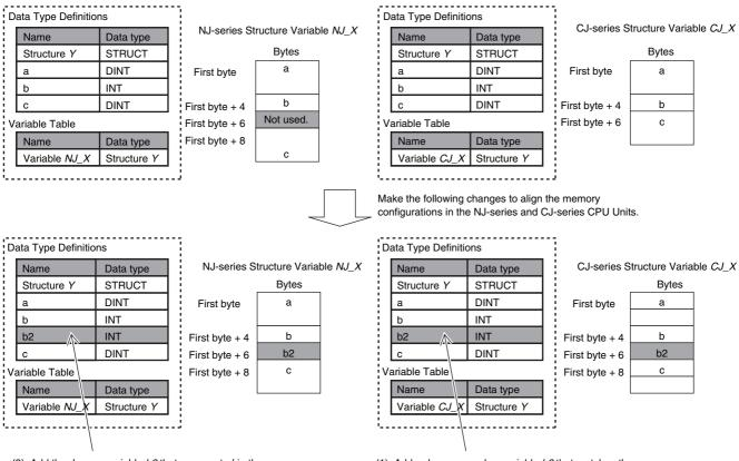
Add a dummy member variable b2 that matches the unused memory location on the NJ-series CPU Unit.
