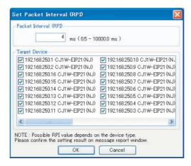
If the packet interval for all connections has been set to the same setting, the dialog box will show that the usage of capacity for the tag data link's allowable communications bandwidth is 76.17% and the fastest set value is 4 ms.
