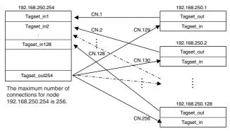
An EtherNet/IP Unit must be mounted to the Controller to increase the maximum number of connections. (Refer to the following figure.)
