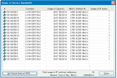
In this case, the tag data link bandwidth that is used by device 192.168.250.10 (Usage of Capacity) also increases (from 33.67% to 50.33%).
