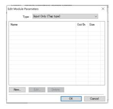
Select Input Only (Tag type) or Input & Output (Tag type) from Type and click the New Button.
