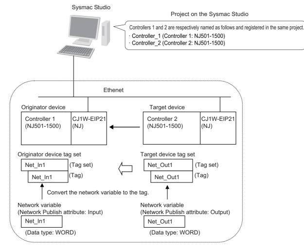
Follow the flow below to set the settings to Controllers 1 and 2 for which to establish EtherNet/IP connections.
