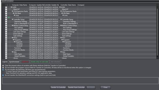
Glear the Do not transfer the EtherNet/IP connection settings (built-in port and Unit) Check Box and click the Transfer to Controller Button.
