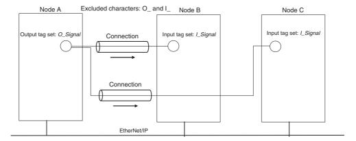
1 Set the same tag set names for the output and input tag sets for the connection. The tag set names can also include forward and backward ellipses.
