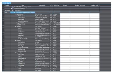
Select the first row listed under the target replacement model CJ1W-EIP21S I/O port and paste the data that you copied from the spreadsheet software.
