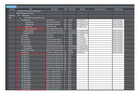
Use the following procedure to transfer the device variables on the CJ1W-EIP21 to the CJ1W-EIP21S. Perform the procedure for all pairs of source and target replacement models, i.e., CJ1W-EIP21 and CJ1W-EIP21S.
