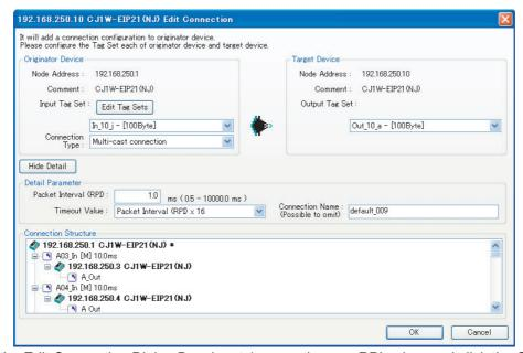
In the Edit Connection Dialog Box, input 1 ms as the new RPI value, and click the **OK** Button. The tag data link bandwidth used by device 192.168.250.1 (Usage of Capacity) increases to 48.67%, which indicates that a RPI is set to a higher speed for this device.
