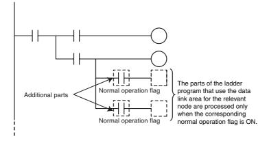
• You can use MC – MCR instructions and JMP instructions to process data only when the data links are operating normally as shown below.
