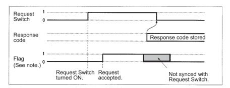
Note The Sending Flag and Receiving Flag will not be changed to TRUE if the high-speed socket service option is selected. Therefore, the program can be controlled only by changing the Send Request Switch and Receive Request Switch to FALSE.
