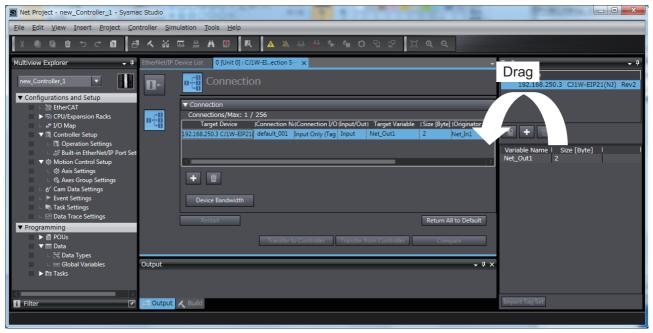
**6** Specify **Originator Variable** and its **Size [Byte]** for the tag set *Net\_Out1* added in step 5. Here, specify *Net\_In1* for **Originator Variable** and 2 for its **Size [Byte]**.
