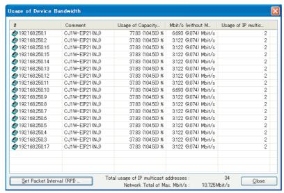
In this case, if there is no multicast filter, the value becomes 104.50%. If there is no multicast filter for an Ethernet switch, communications errors may occur depending on the communications load of the EtherNet/IP Unit.
