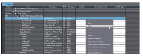
The variables, variable comments, and variable types are set for the target replacement model CJ1W-EIP21S.
