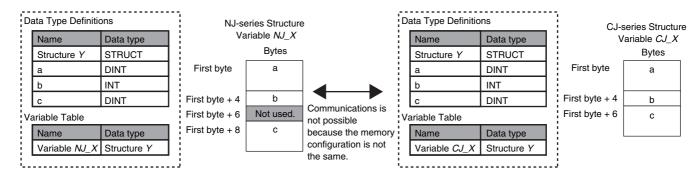
To align the memory configurations in the NJ-series and CJ-series CPU Units, offsets are set in the Sysmac Studio.
