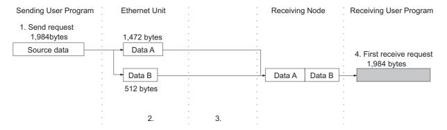
As shown above, the UDP protocol handles data communications as datagrams, so that the send data is restored to the original data before being passed to the user program.
