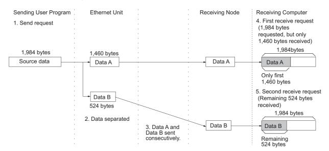
When using TCP protocol, the fragmented data is passed to the user program.
