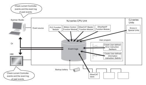
To use an HMI to check events, connect the HMI to the built-in EtherNet/IP port on the CPU Unit.
