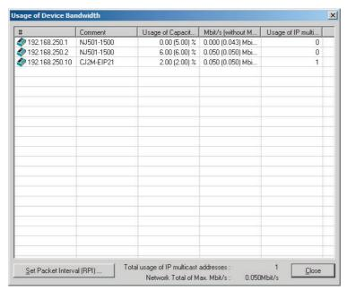
The *Usage of Capacity* (without multicast filter) column will show the percentage of the allowed tag data link bandwidth being used, and the *Mbit/s* (without multicast filter) column will show the network bandwidth being used.
