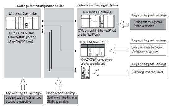
Use the Network Configurator if a CS/CJ-series PLC operates as the originator device.
