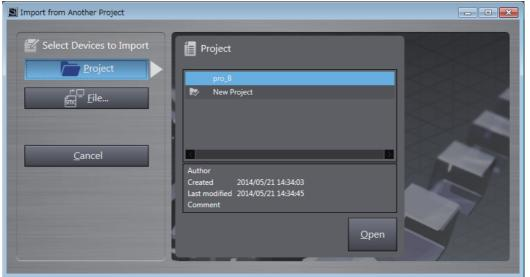
(3) The list of EtherNet/IP devices registered in the selected project will be displayed. Select the target devices to import, and click the Import Button.
