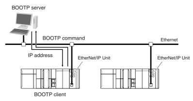
The EtherNet/IP Unit IP address is obtained from the BOOTP server when the power is turned ON.
