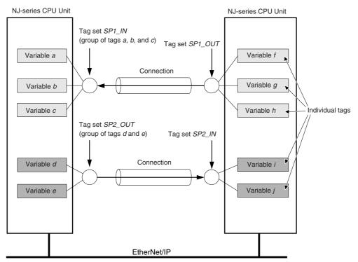
Note To enable a connection, each tag set must include only input tags or only output tags. (Both input and output tags cannot be included in the same tag set.)
