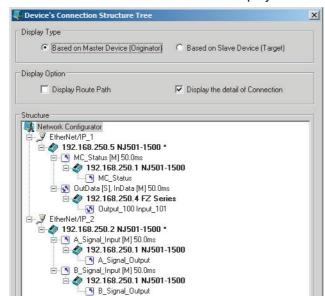
**4** A device connection structure tree is displayed when processing is completed.
