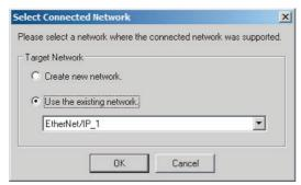
The Network Configurator will connect to the EtherNet/IP network. If the Network Configurator goes online normally, "On-line" is displayed in the status bar at the bottom of the window.
