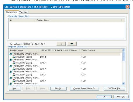
Information about the connection with device 192.168.250.10 is registered in the Register Device List. Double-click this connection to edit the settings.
