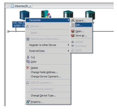
Click the Tag Sets Tab at the top of the Edit Device Parameters Dialog Box. There are two kinds of tag sets: input (consume) and output (produce).
