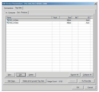
To place more than one input variable (input tag) imported from the Sysmac Studio into one tag set, you must delete the input tags that were registered. Select the tag set containing the variables you want to put into a tag set, then click the **Delete** Button. A confirmation dialog box is displayed to confirm that you want to delete the selected tag set and the tags contained in that tag set. You only want to delete the tag set, so click the **No** Button.
