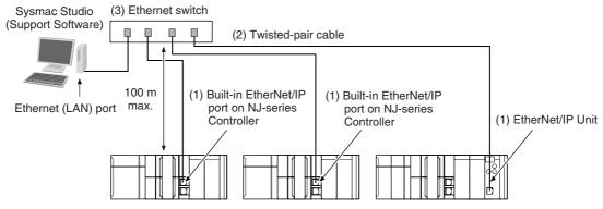
EtherNet/IP System Configuration Example
