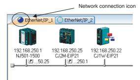
Select Network - Change Connect Network to switch the connected network.
