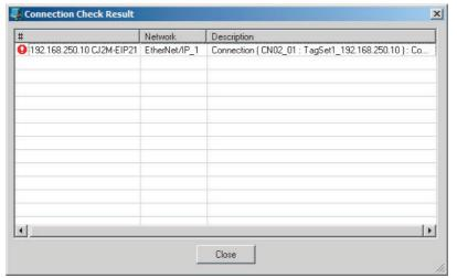
If an inconsistency is found, open the originator's Edit Device Parameter Dialog Box and click the **Connection** Tab. The inconsistent connection in the Register Device List is displayed with a icon (instead of the normal icon). To change the connection setting and select a different target variable, select the connection as shown below and click the **Edit** Button.
