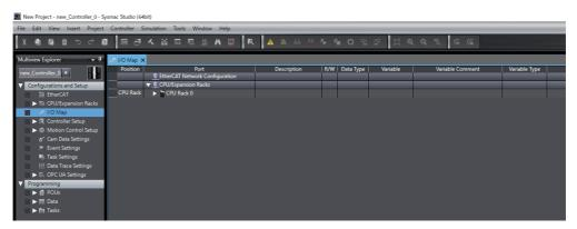
2 In the I/O Map Tab Page, right-click the source replacement model CJ1W-EIP21 and select Expand/Collapse All.
