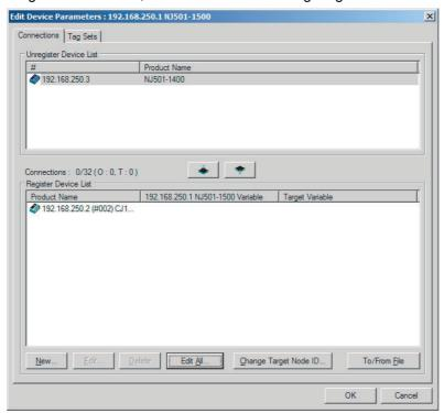
Target node IDs are assigned to the devices that are registered in the Register Device List.
