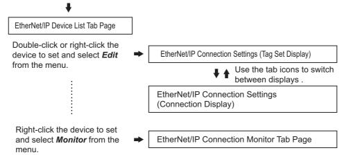
· Transferring connection settings to the Controller from the computer
