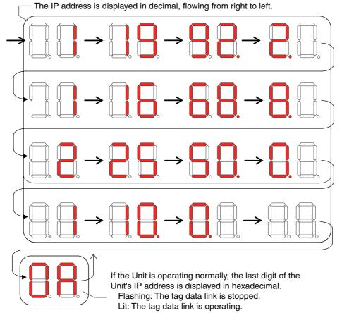
If an error occurs, the error code will be displayed alternately with the rightmost byte of the affected device's IP address. For details on error codes, refer to Section 15 Troubleshooting.
