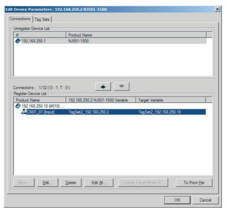
(4) The device's Edit Connection Dialog Box will be displayed. Input a new packet interval (RPI) value, and click the OK Button.
