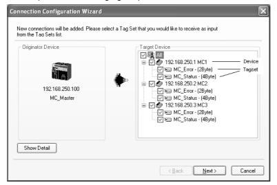
**4** A list of tag sets is displayed on the right side of the Wizard Dialog Box with target devices that support receiving input data.
