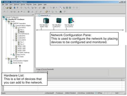
To manage two or more networks, you can select **Network** – **Add** to add a new Network Configuration Pane. You can add a new Network Configuration Pane.
