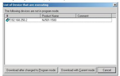
If the **Download after changed to Program mode** Button is clicked, all CPU Units are changed to PROGRAM mode and the parameters are downloaded. Confirm safety for all controlled equipment before you change the CPU Units to PROGRAM mode. You can restore the operating modes after the parameters are downloaded.
