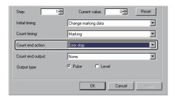
11 Select "A" as the location from which to output an I/O signal when the end value of the counter is reached, under [Count end output].
