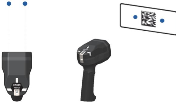
The aiming dots are smaller when the V460-H is closer to the symbol and larger when it is farther from the symbol. Scan symbols with smaller bars or elements (mil size) more closely, and those with larger bars or elements (mil size) more distantly.
