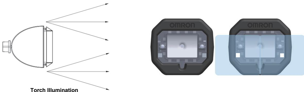
Torch Illumination cannot be used in combination with Dome Illumination or Low Angle Illumination. Torch Illumination uses high-intensity white LEDs only.
