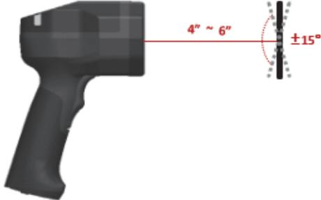
*Start at approximately 4" ~ 6" ( $\pm 100\text{mm} \sim 150\text{mm}$ ) and, if necessary, tilt the part ( $\pm 15^\circ$ ).*
