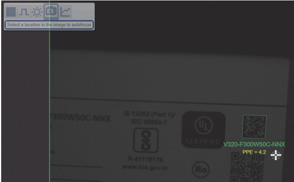
**Note:** If you click the **Autofocus** button to the left of the **Spot Focus** button, the handheld will switch from Spot Focus to regular Autofocus functionality. If the handheld is in **Triggered** mode, only the Spot Focus icon will appear.
