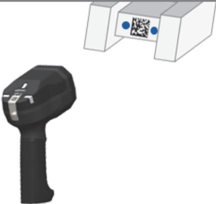
*Use the two LED dots to positioning the code.*
