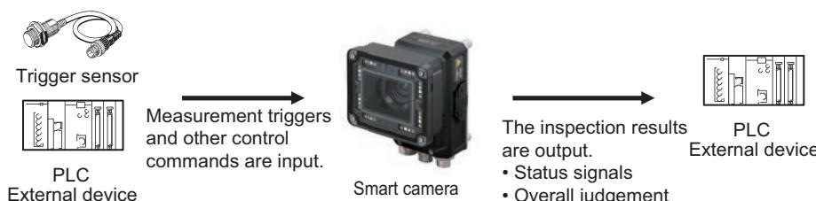
The following methods are used to exchange commands and data, between an external device and the smart camera.
