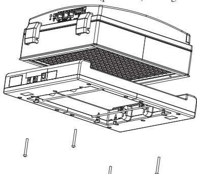
Insert the nuts into the remaining four mount holes.
