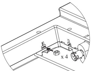
Install the Air Clean Ionizer using the four M4x35 screws (provided) at a tightening torque of 1.2 to 1.6 N.m.
