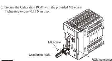
pushing in or pulling out the calibration ROM, be sure to turn off the power of the Sensor Controller. Otherwise, a failure might be caused
