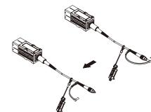
(2) Connect the fiber cable and calibration ROM with the Sensor Controller. Mount the fiber cable in the direction where the protruding portion of the fiber connector and the groove portion of the fiber adapter are aligned. Align the groove portion of the fiber adapter with the protruding portion of the fiber connector, and rotate the screw portion clockwise while pushing it.
