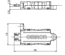
\* Included in the Sensor Head (ZW-S7010/S7020/S7030/S7040). Be sure to use the Sensor Head and Calibration ROM of the same serial numbers.
