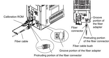
Grip the bush portion of the fiber cable (black) on the right-hand figure, align the groove portion of
