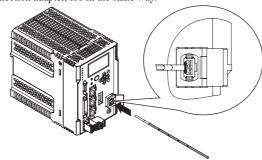
(3) Cleaning of the end face of the fiber connector of the sensor head side Remove the cap of the fiber connector, and wipe up and down the end face of the fiber connector around three times. Clean around the two guide pins as well.
