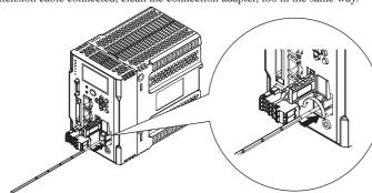
(3) Cleaning of the end face of the fiber connector of the sensor head side Remove the cap of the fiber connector, and wipe up and down the end face of the fiber connector around three times.
