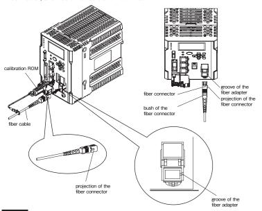
e cable cannot be connected properly by holding the bush portion of the fiber connector · Not inserting the connector to the end will result in failure of light signal transmission and erroneous measurement.
