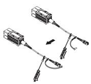
(2) Connect the fiber cable and calibration ROM with the sensor controller. When connecting a fiber cable, grip the fiber connector and align the groove portion of the fiber adapter of the sensor controller with the protruding portion of the fiber connector, and insert the cable until it clicks.
